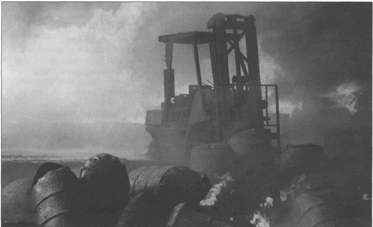
**Figure 5:** Fork-lift truck caught in the inferno in J-Bay, and burst metal drums in the foreground. Courtesy of West Yorkshire Fire Service.
