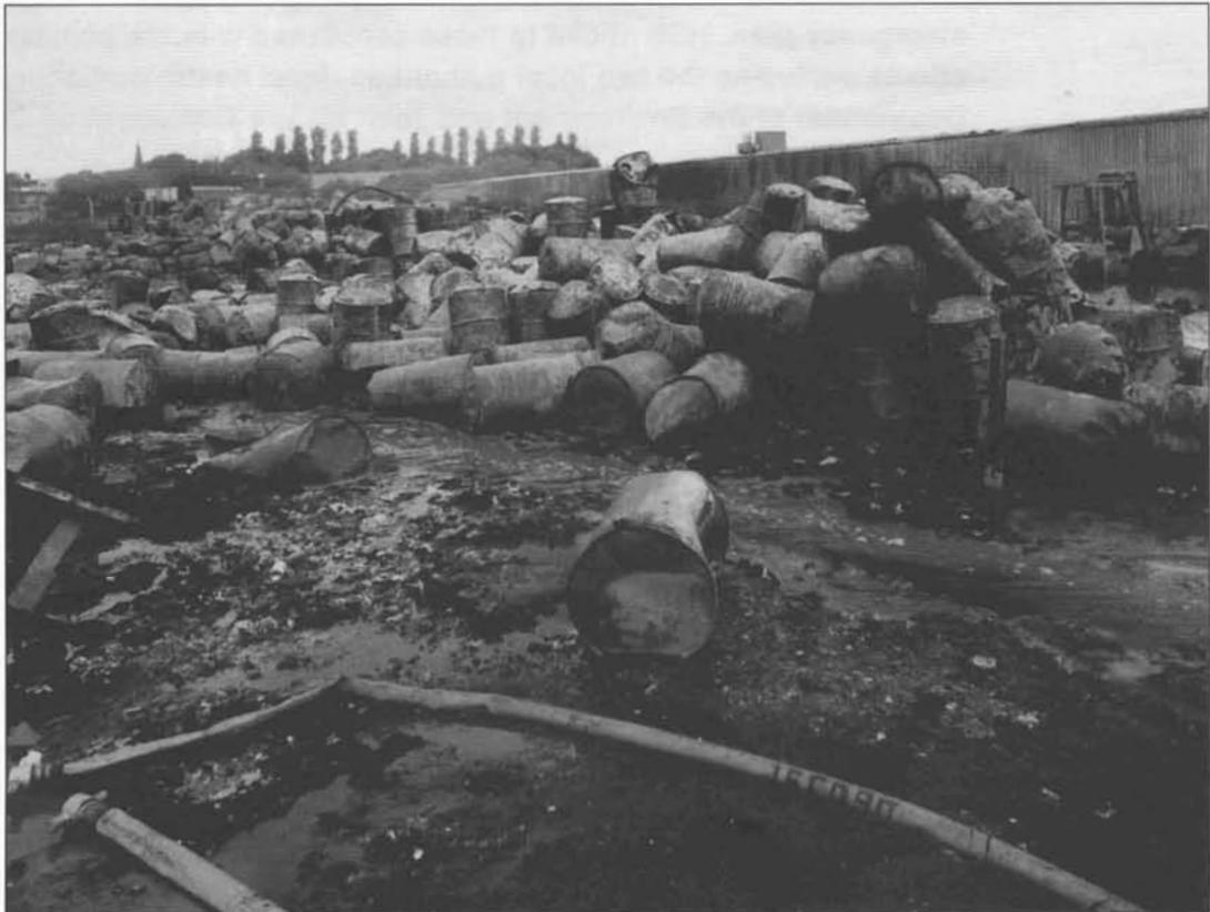
**Figure 14:** Drum storage areas at X and J-Bays looking towards finished goods warehouse. Contaminated water can be seen flowing from the area.
