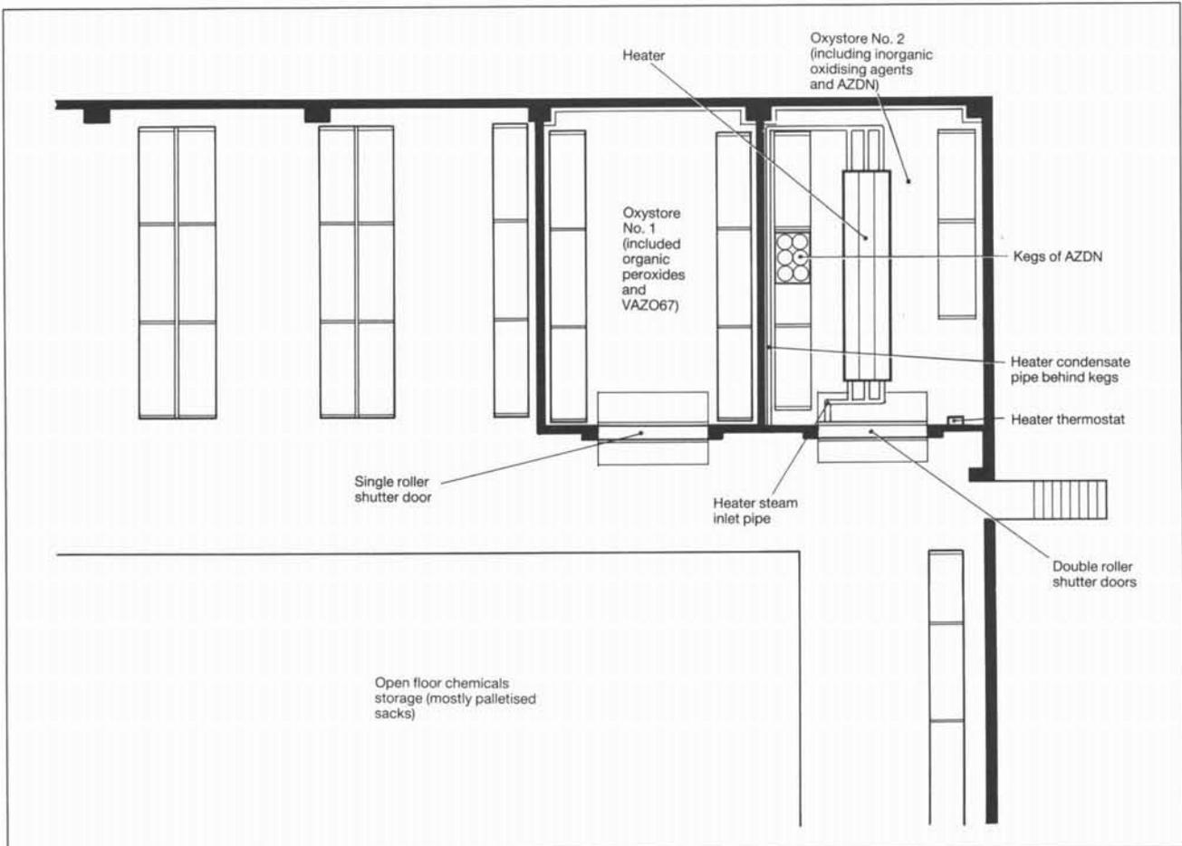
**Figure 15:** North east corner of raw materials warehouse.
