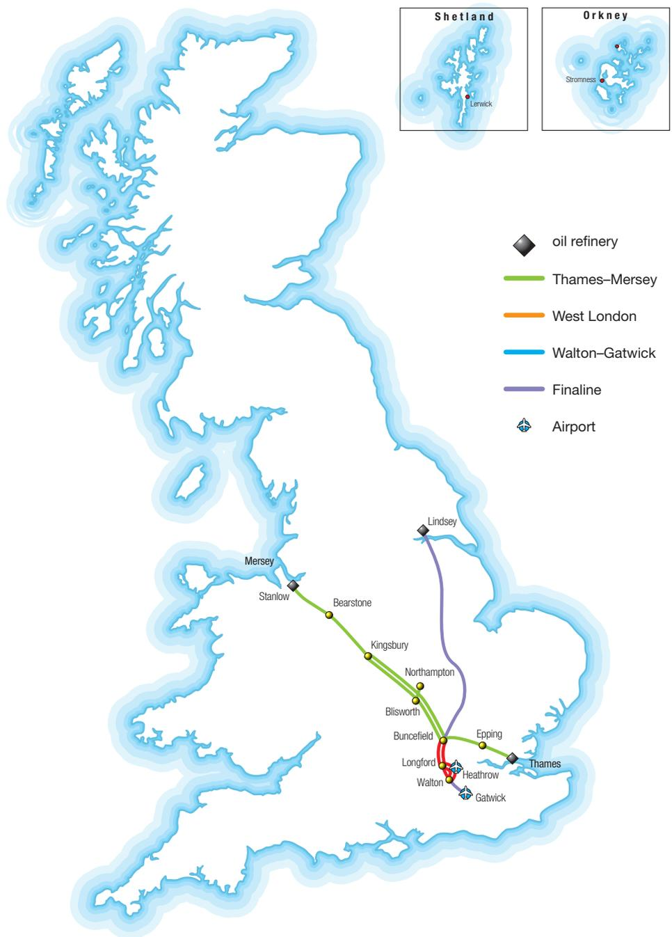
Figure 4 Schematic showing the pipeline system supplying Buncefield
