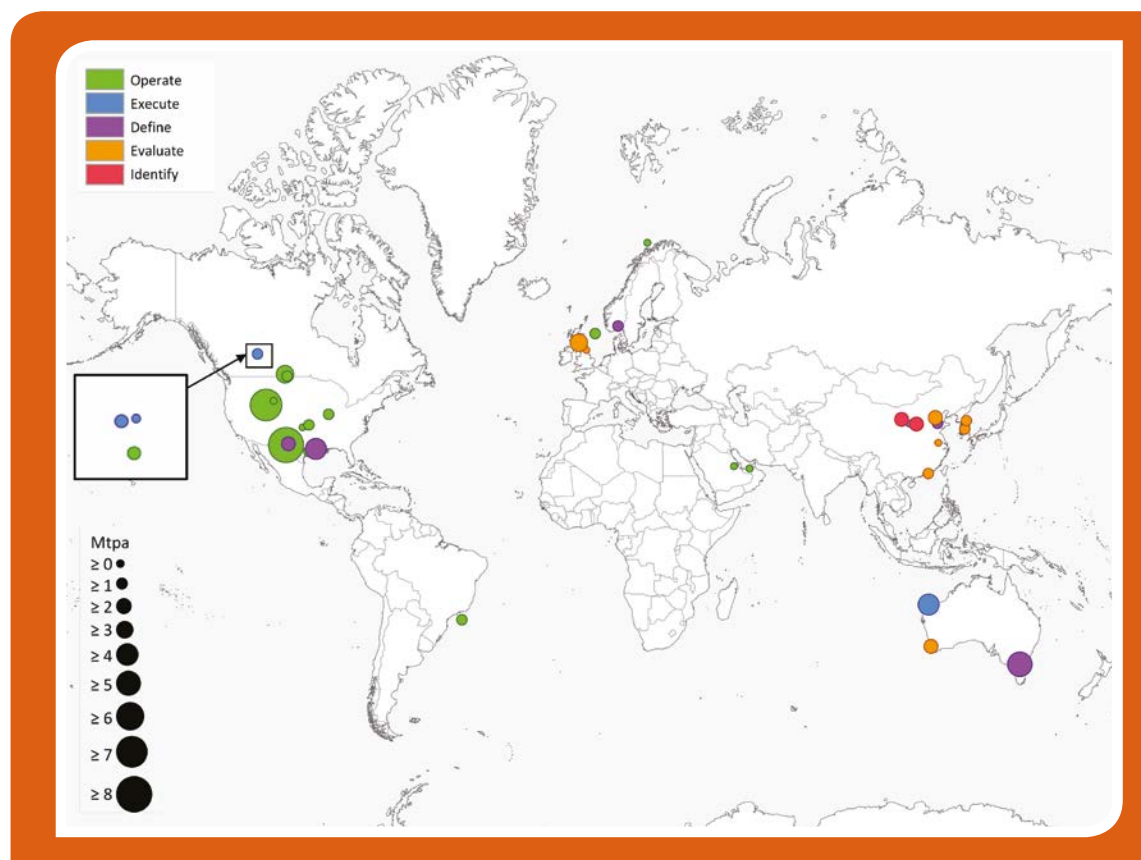
Figure 3. Large-scale integrated CCS projects under development or operational around the world and lifecycle stage. Circle size is proportional to the CO 2 capture capacity of the project (million tonnes per annum, Mt pa). Data from the Global CCS Institute.
