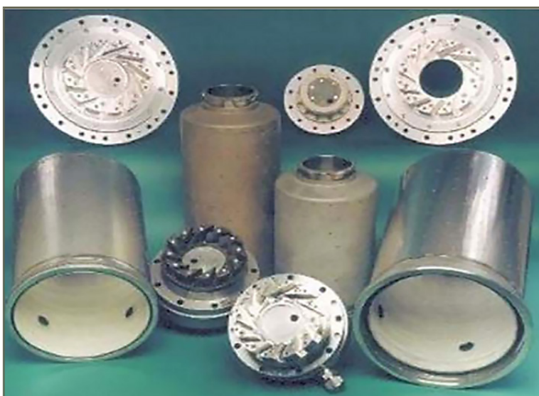
Figure 2: DLE (Lean pre-mix) combustion cans and fuel injectors (1990s) to present.
