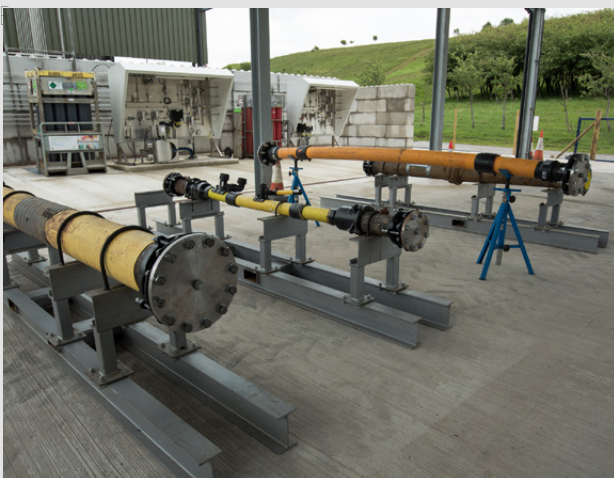
Phase 1 - Various configurations of gas network assets assembled for testing at the bespoke facility based at the Health and Safety Executive's Science Division, in Buxton, Derbyshire.
