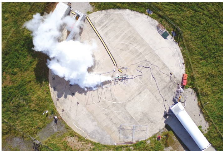
Testing: Still of controlled liquid hydrogen spill from a tanker, performed on HSE's site in Buxton. Images captured from drone video recordings.
