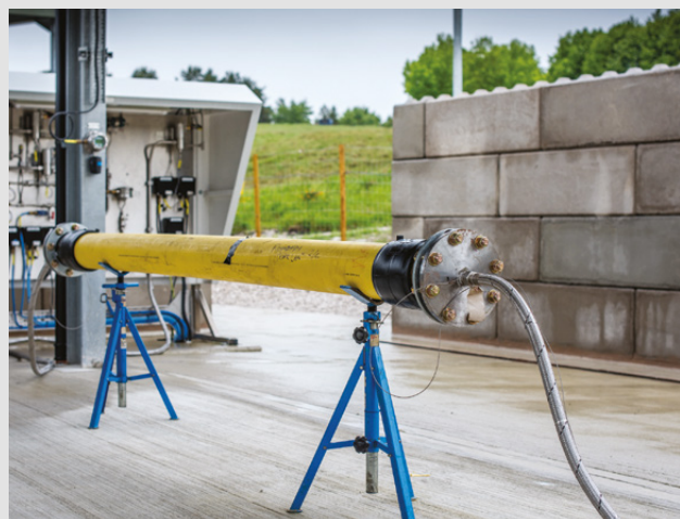
Phase 1 - Various configurations of gas network assets assembled for testing at the bespoke facility based at the Health and Safety Executive's Science Division, in Buxton, Derbyshire.
