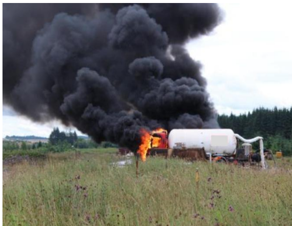
Figure 2- Fully engulfed cab and diesel pool fire under vehicle
