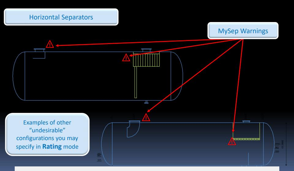
INFO: The selected orientation of demisting device #1 typically results in gas maldistribution. Local overloading of this device may occur and performance may be lower than predicted. CFD verification is recommended.
