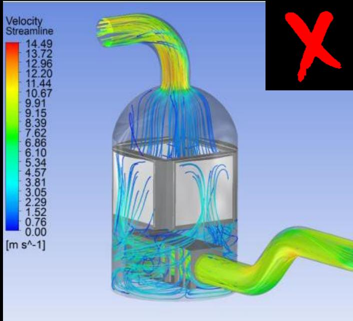
LNG process – carry-over at 35% capacity
