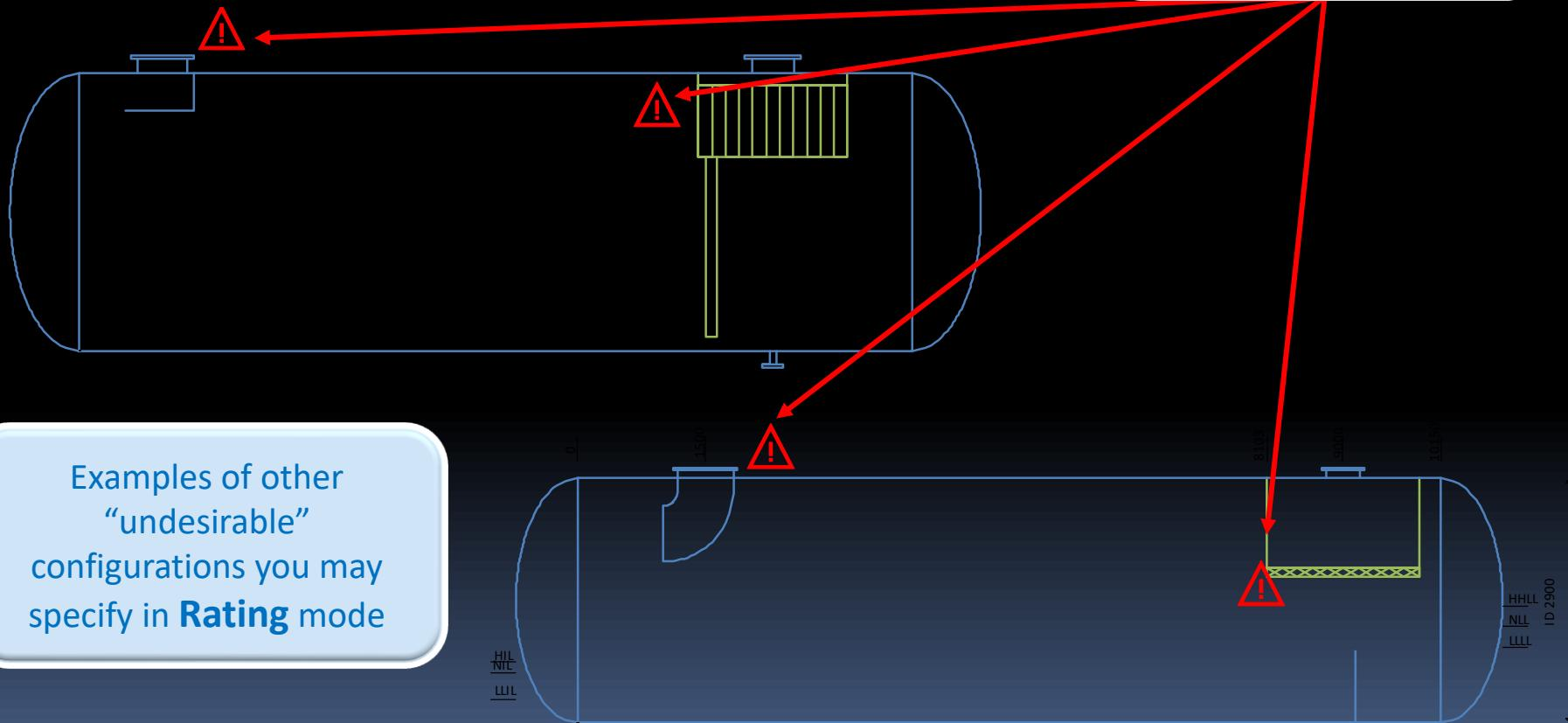
**INFO:** The selected orientation of demisting device #1 typically results in gas maldistribution. Local overloading of this device may occur and performance may be lower than predicted. CFD verification is recommended.
