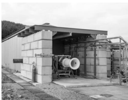
Figure 1. Rolls-Royce Viper Type 301 jet engine modified to run on liquid butane
