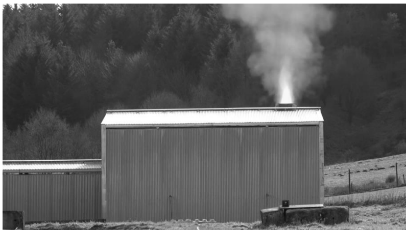
Figure 9. Flame emerging from exhaust duct during a test with the end plate on
