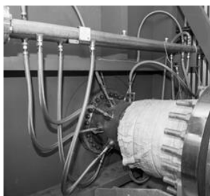
Figure 4: Radially arranged fuel and oxygen injection tube system.
