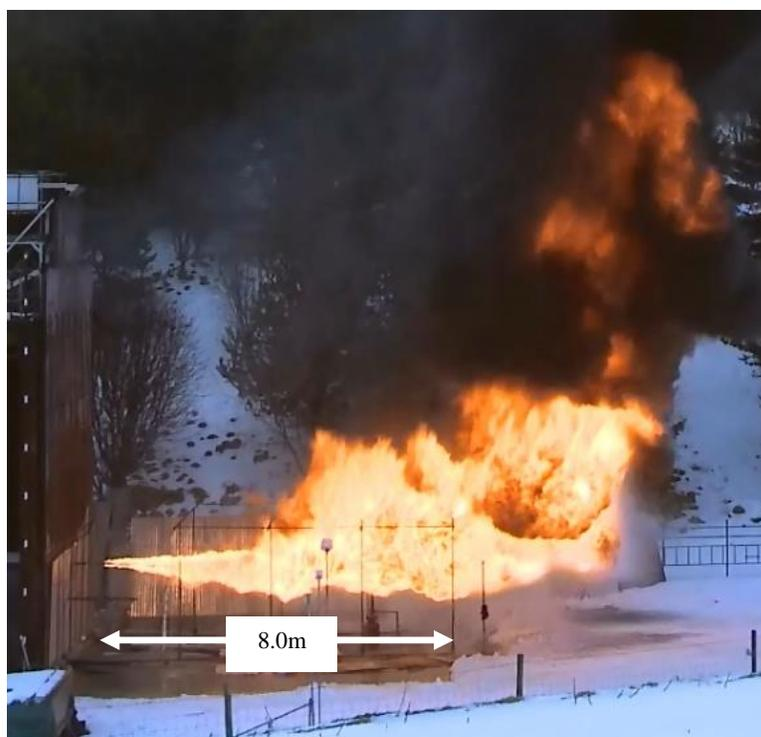
Figure 3: Liquid solbit jet fire SC22 (S:B =1.4, 1.47 kg/s)
