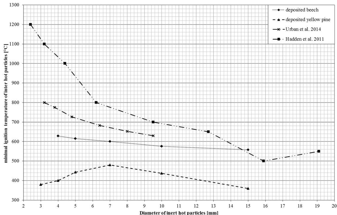
Figure 8: Comparison of results of deposited dust layers and the investigations of (Urban et al. 2014) and (Hadden et al. 2011)
