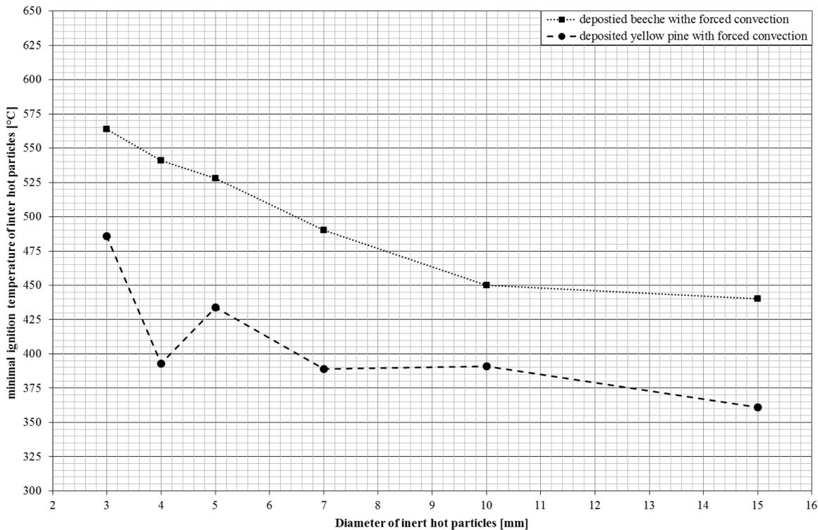
Figure 5: results of the Experimental Ignition Test of inert hot particles for deposited dust layers with forced convection (cf. Tessororf 2017)
