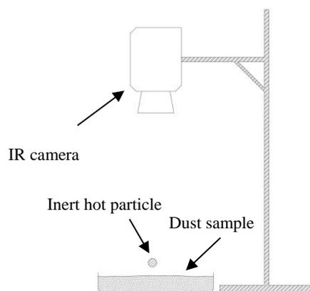
Figure 2: Scheme of the experimental setup for deposited dust layers (cf. Bechem et al. 2016)
