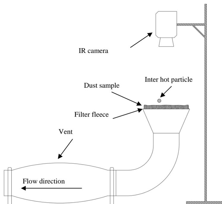
Figure 3: Scheme of the experimental setup for deposited dust layers with forced convection (cf. Bechem et al. 2016)
