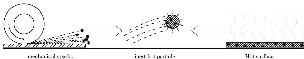
Figure 1: Scheme of the inert hot particle Model
