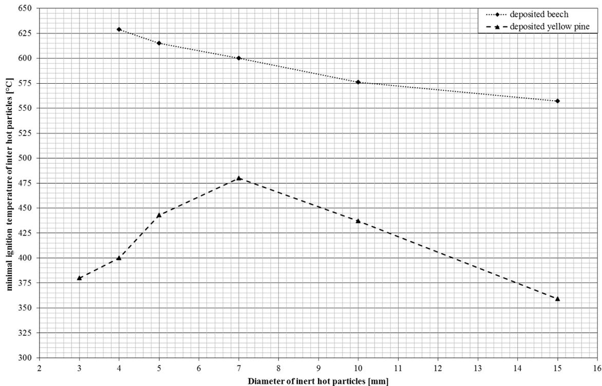
Figure 4: results of the Experimental Ignition Test of inert hot particles for deposited dust layers
