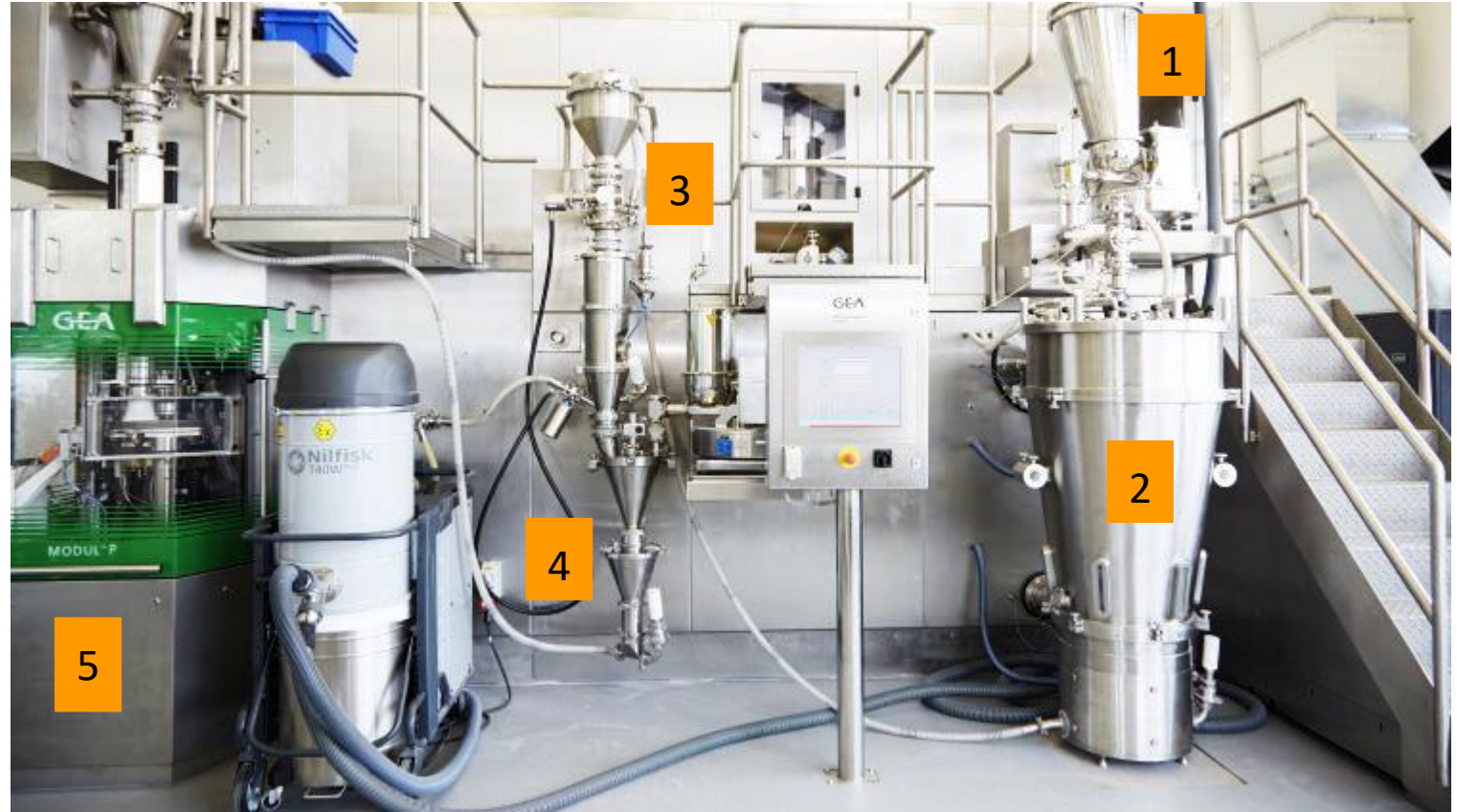
1: Twin screw granulation 2: Fluid bed dryer 3: Cone mill 4: Blender 5: Tableting machine
