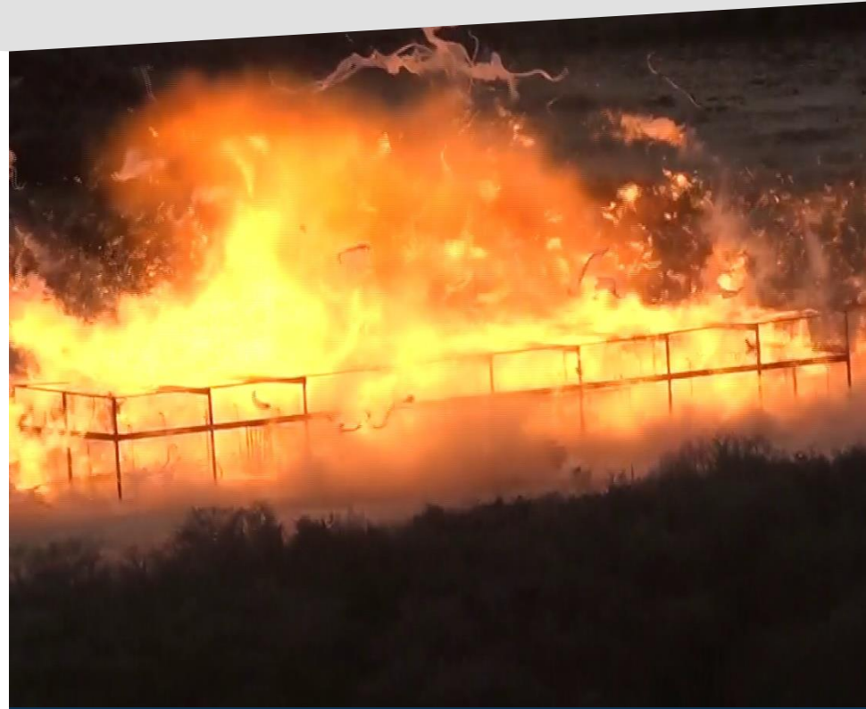
Large Cloud VCE Test at BakerRisk's BCTF
