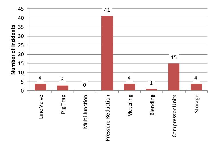
Nearly 60% of the incidents from Pressure Reduction units, even though Pressure Reduction units make up less than 25% of the population
