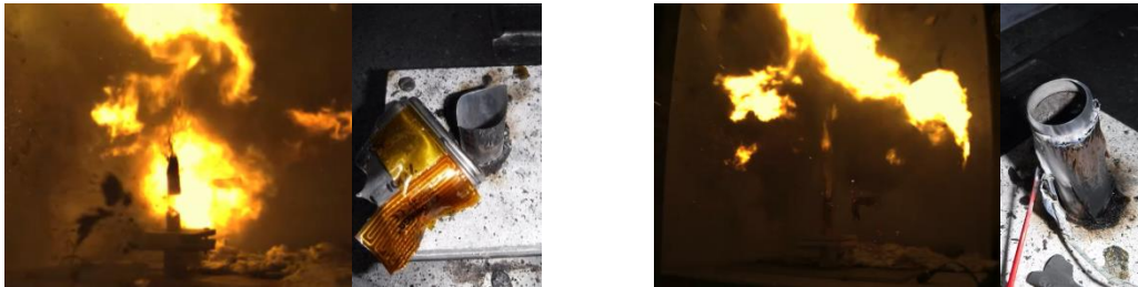
Figure 7 The projected fireballs captured on the high speed camera during cell type 2 failure, showing the cell being split in two and the after photo (left) and another typical projected fireball and the after photo (right)
