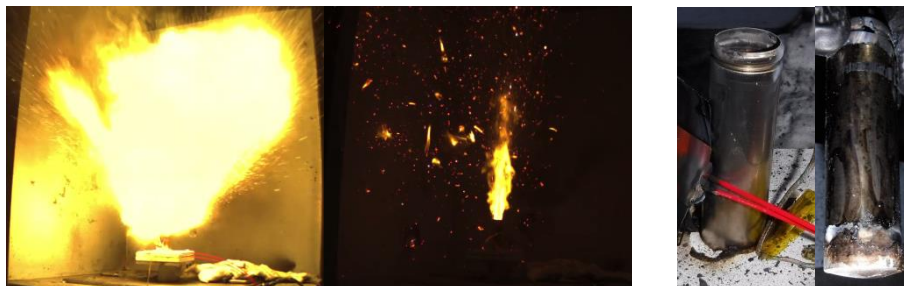
Figure 8 The aggressive jet flame captured on the high speed camera during cell type 3 failure and the ejection of molten metallic particles (left), and the cell after the test (right)
