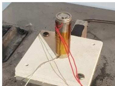
Figure 1 The 5 kg load cell set up
