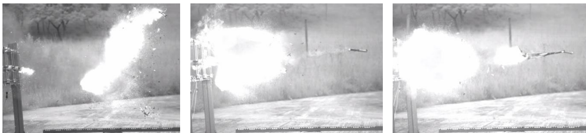
Figure 13 Screenshots from the high speed camera showing the initial projection of cells 1 (left), 2 (middle) and 3 (right)
