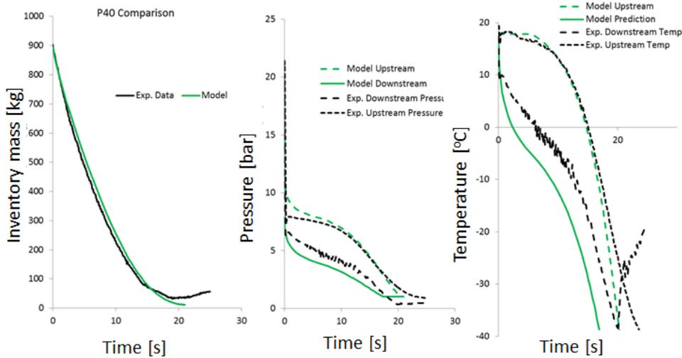
**Figure 7** Comparison of PiRRaM to Isle of Grain experiment P40, from left to right, Inventory mass, Pressure and Temperature
