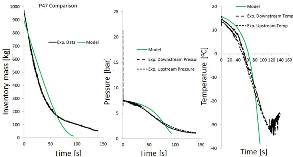
**Figure 8** Comparison of PiRRaM to Isle of Grain experiment P47. The model predictions for the upstream and downstream temperature and pressure are indistinguishable, and the model line therefore represents both.
