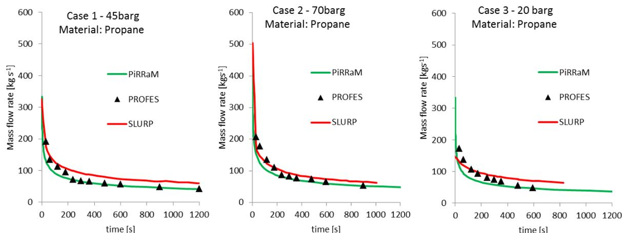
**Figure 3** Comparison of the transient mass flow rate for the predictions described in Clever *et al.* (2003) (SLURP and PROFES) and PiRRaM, for releases of propane from a 25 cm diameter pipe at 45 barg (left), 70 barg (middle) and 20 barg (right).
