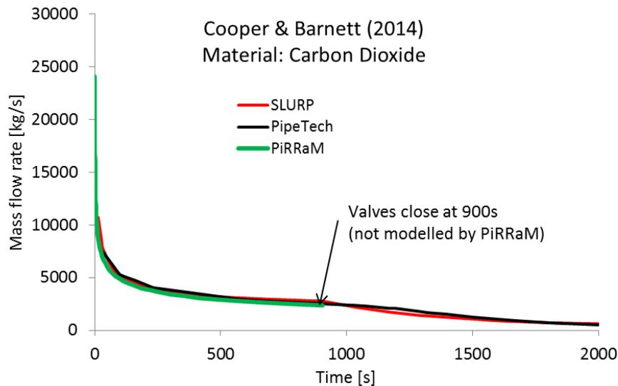
**Figure 6** Predictions of the mass flow rate versus time from PiRRaM, PipeTech and SLURP for a full-bore breach to a 96 km long pipeline transporting carbon dioxide.
