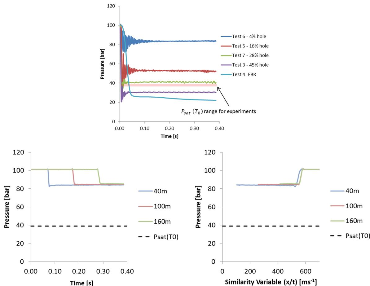
**Figure 1** Pressure versus time at a position 250 mm upstream of the orifice plane for 5 of the CO<sub>2</sub>PipeTrans Phase 3 experiments (top), pressure profiles in the pipe for a 10 mm diameter hole (CO<sub>2</sub>PipeTrans-P3T6) at various locations upstream of the orifice against time (lower left), and the corresponding profiles shown using the Landau and Lifschitz (1987) similarity theory (lower right).
