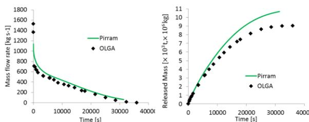
**Figure 4** Comparison of PiRRaM and OLGA predictions for the mass flow rate and released mass.
