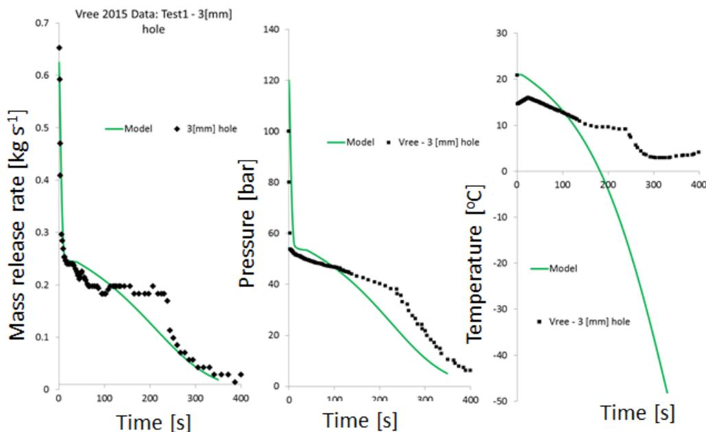
Figure 11 Comparison of PiRRaM to the Vree *et al.* (2015) Test 1 experiment (3 mm hole)
