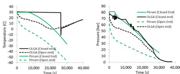
**Figure 5** Comparison of PiRRaM and OLGA predictions for the temperature and pressure at the open and closed ends of the pipe.
