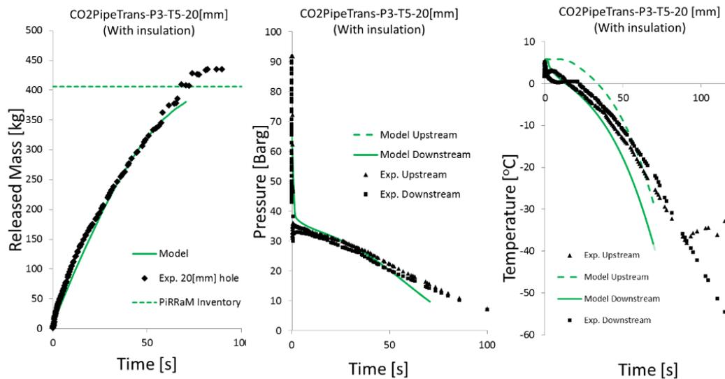
**Figure 9** Comparison of PiRRaM to the CO<sub>2</sub>PipeTrans Phase 3 Test 5 experiment (20 mm hole)
