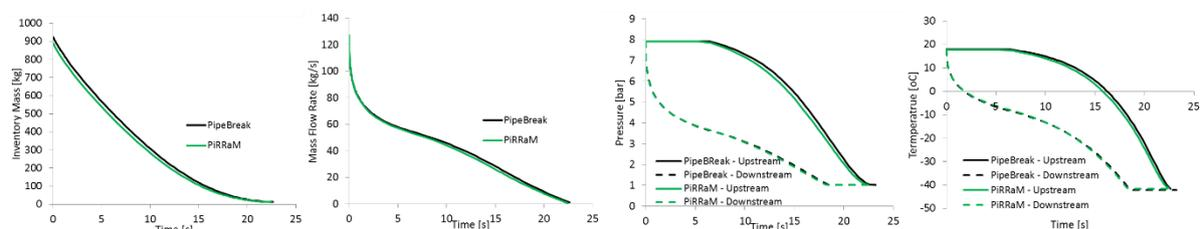
**Figure 2** Comparison between PiRRaM (green lines) and DNV's PipeBreak model in Phast (black lines) for the Isle of Grain P40 trial assuming a saturated initial condition showing inventory mass (far left), mass flow rate (middle left), upstream and downstream pressure (middle right) and temperature (far right) respectively.
