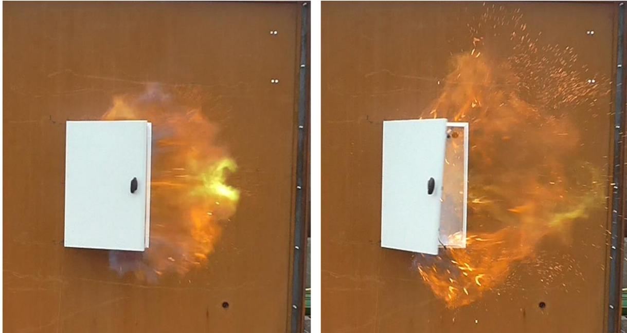
Figure 10 - front view of venting flame shape in test 3; frame interval 20 ms
