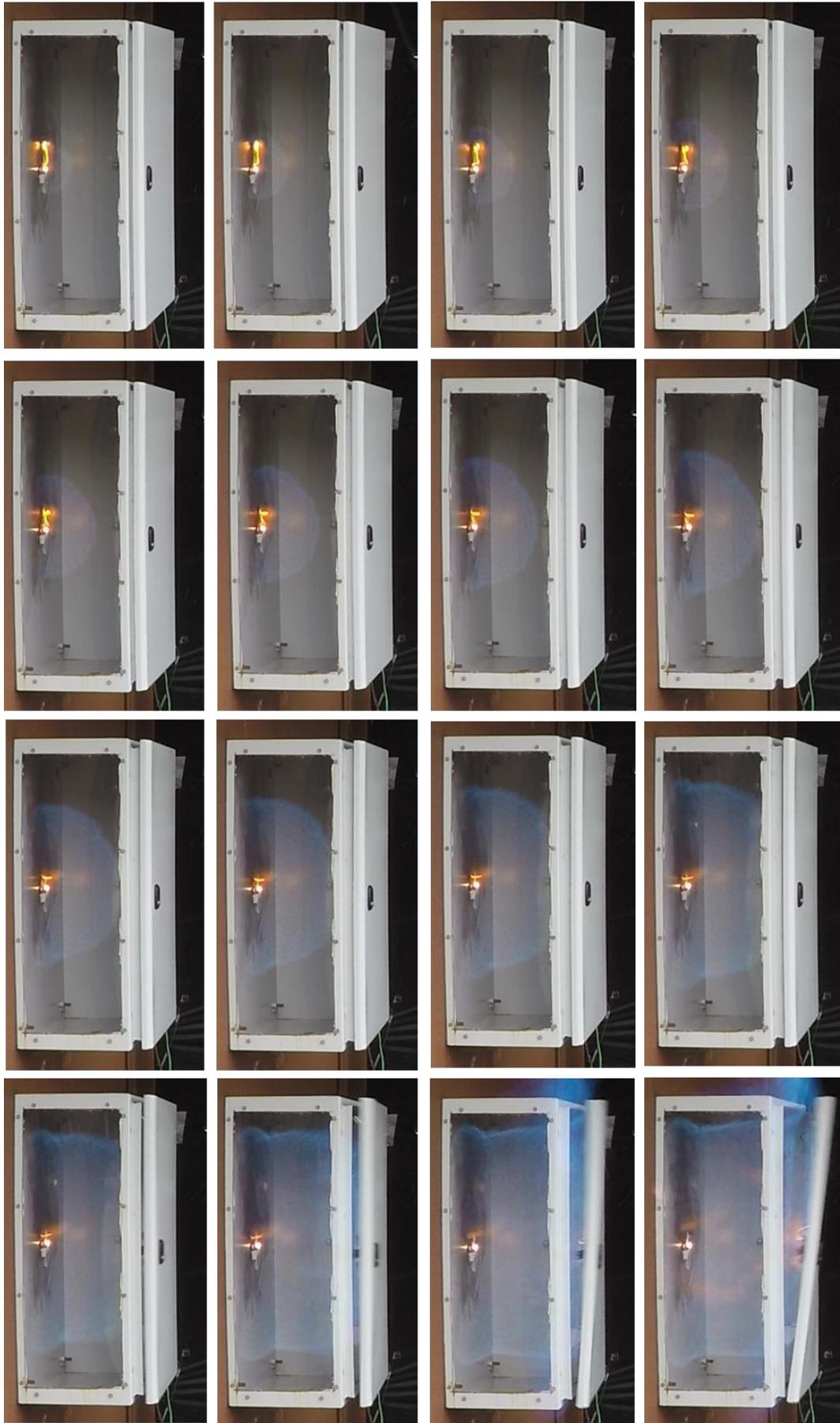
Figure 9 - Flame development in test 4; frame intervals 4.17 ms
