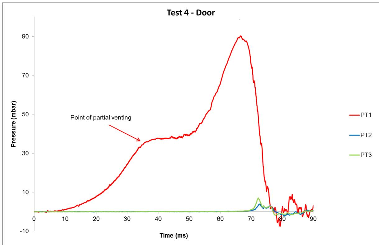
Figure 5 - Pressure trace for test 4
