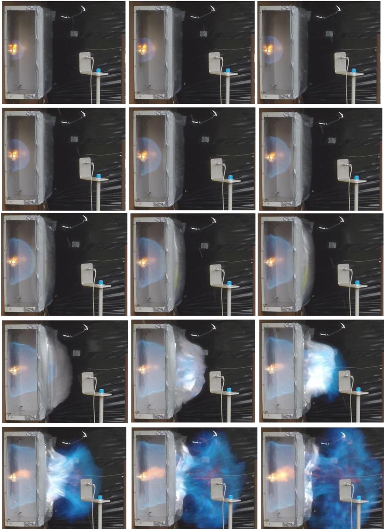
Figure 6 - flame development in test 1; frame intervals 4.17 ms
