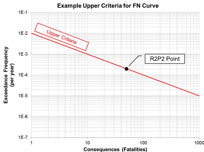
Figure 11: Example Upper Criteria for FN Curve
