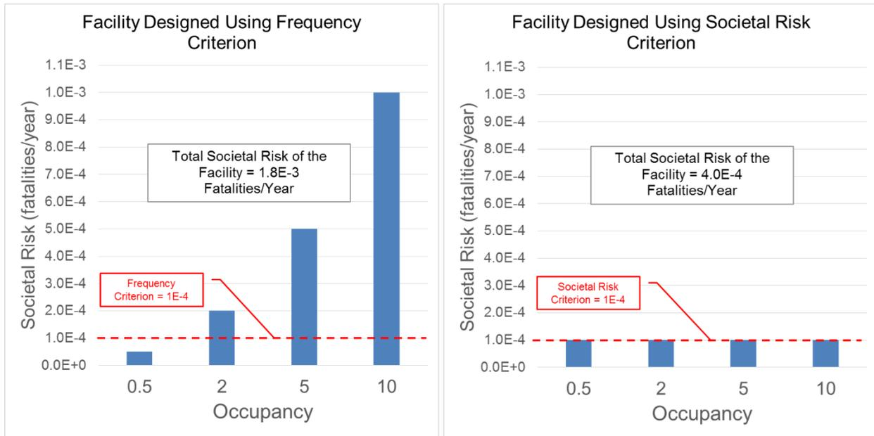
Figure 10: Difference in Using a Frequency Criterion and Societal Risk-Based Criterion in Building Design on the Overall Risk of a Facility
