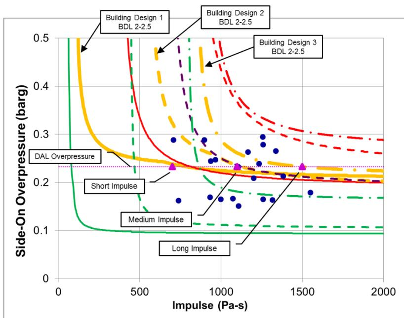
Figure 6: Example 1 – P-i Blast Scatter Plot for Three Building Designs of the Same Construction Type
