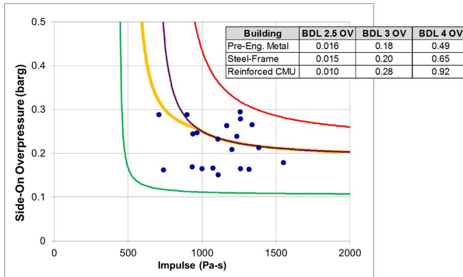
Figure 8: Example 2 – P-i Blast Scatter Plot for Three Identical Building Designs Constructed with Different Materials
