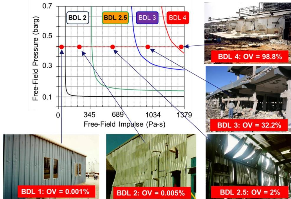
Figure 2: Example Pressure-Impulse Diagram and BDLs for same Overpressure and Different Impulses (Durations)
