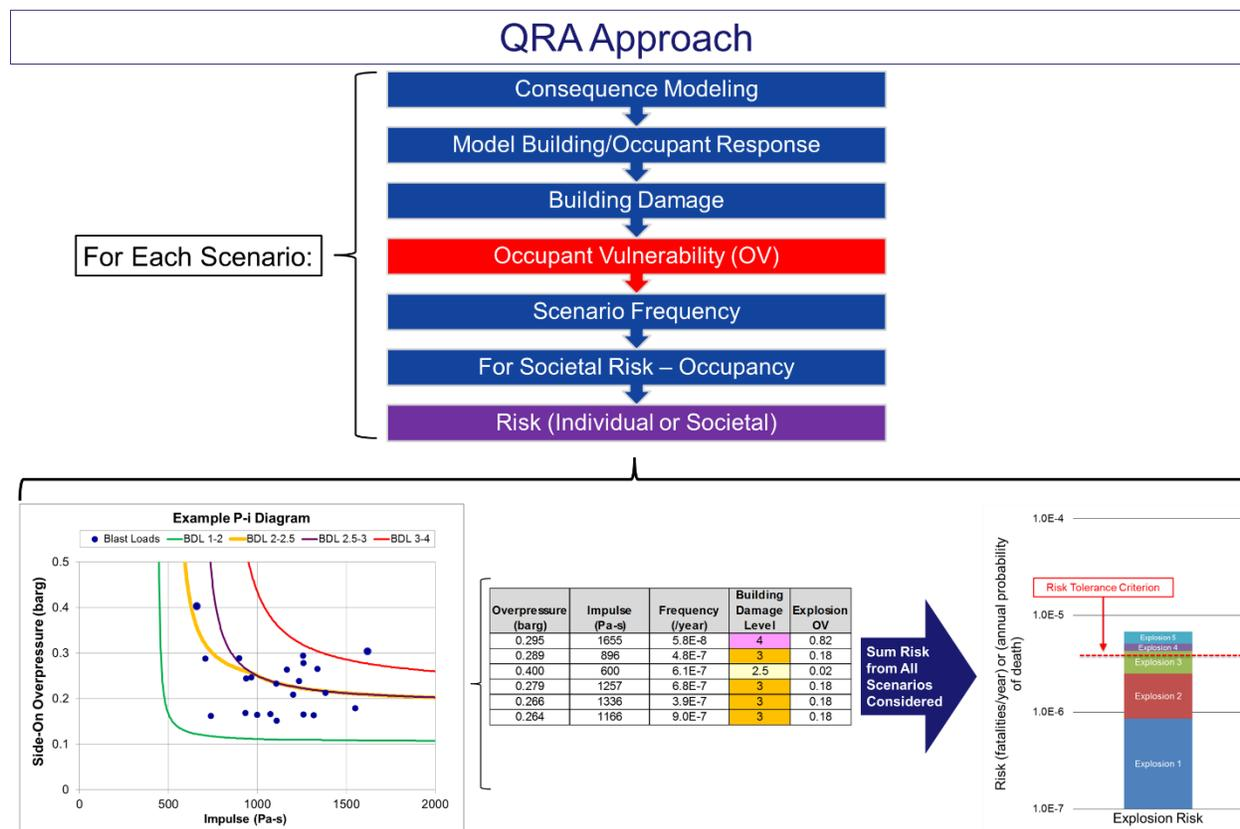
Figure 4: Schematic of QRA Approach
