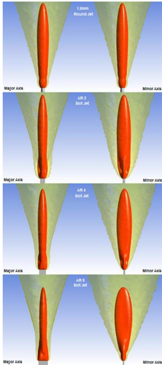
**Figure 4** Isosurfaces at the lower and upper flammability limits of hydrogen, yellow (2% v/v) and red (74% v/v) respectively, for the considered nozzle shapes. From top to bottom: round jet, rectangular nozzle aspect ratio = 2, 4 and 8
