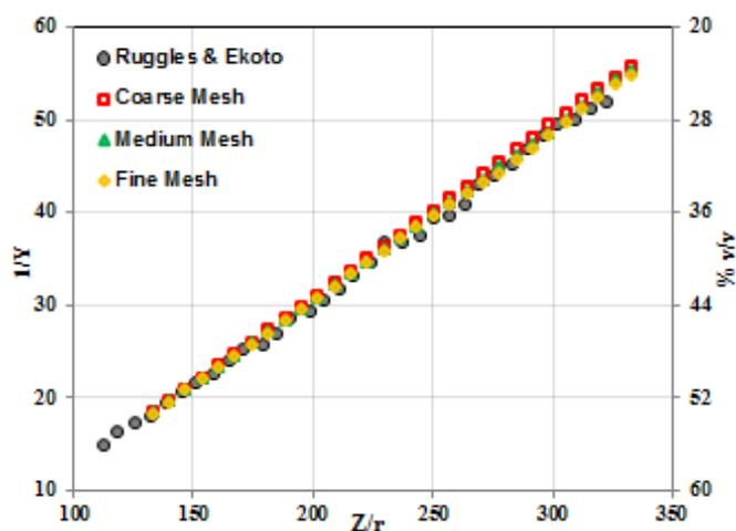
**Figure 1** Comparison of the experimental (Ruggles and Ekoto, 2012) and CFD results for the inverse hydrogen mass fraction against normalised axial distance
