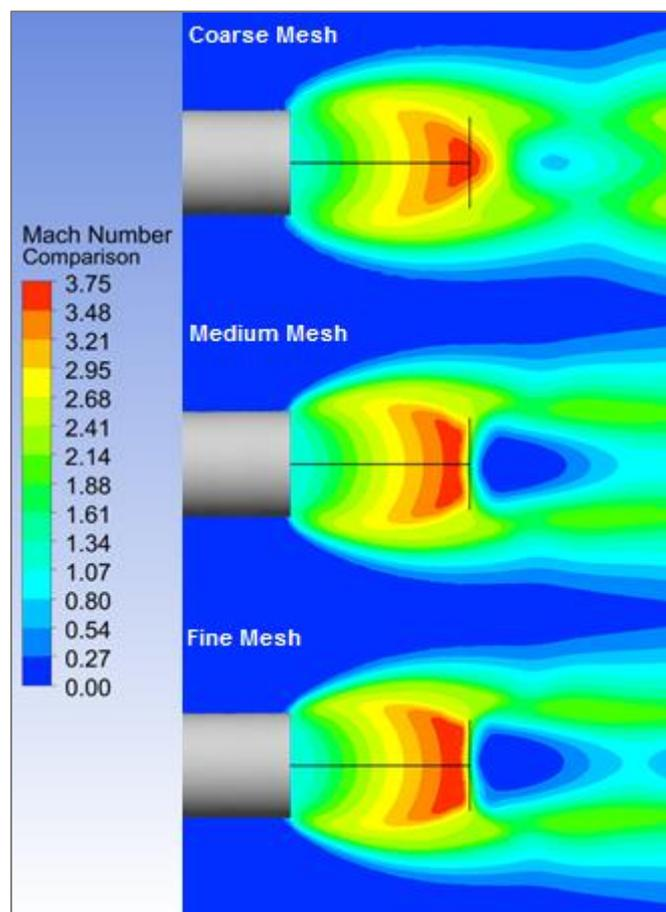
**Figure 2** Comparison of barrel shock region and Mach disk resolution for different computational meshes
