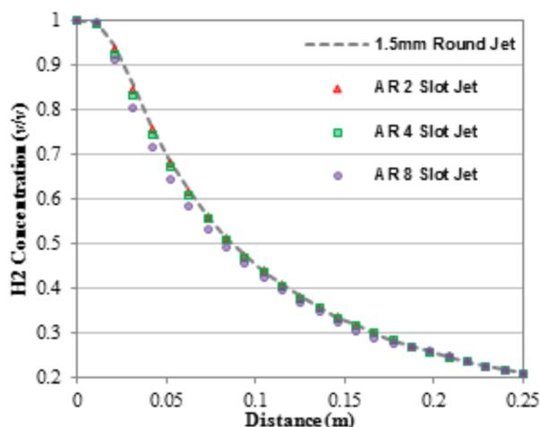
**Figure 6** Centreline axial hydrogen concentration profiles for the four considered nozzle shapes
