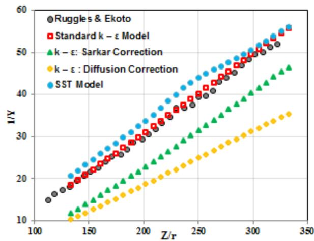
**Figure 3** Comparison of the experimental (Ruggles and Ekoto, 2012) and CFD turbulence model sensitivity results for the hydrogen concentration against the axial distance
