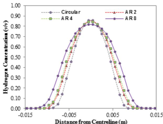
**Figure 5** Radial hydrogen concentration profiles across the nozzle minor axis for the four considered nozzle shapes at a distance of 0.03 m downstream of the nozzle. Here AR 2, 4 and 8 represent rectangular nozzles with aspect ratio = 2, 4 and 8 respectively
