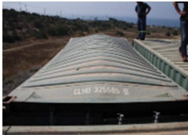
Figure 6 – Deformed container 5 July 2011
