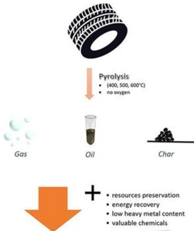
Figure 2: Pictorial representation of tyre conversion in the pyrolysis process.
