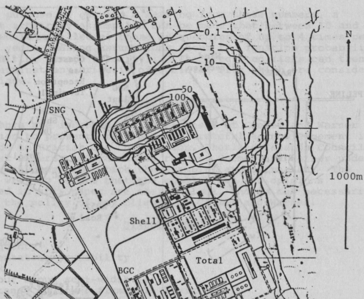
Figure 4 Risk contour plot for 0.3 bar explosion overpressure risk (per million years) for St. Fergus coastal gas reception terminal.
