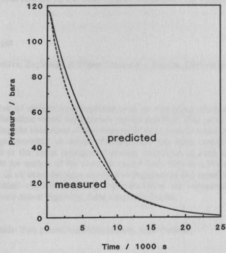
Figure 13 Pressure at intact (MCP-01) end of line
