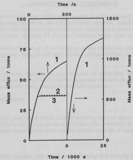
Figure 14 Total mass efflux out of ruptured (Piper) end of line: line 1 refers to case 1, line 2 to case 2 and line 3 to case 3
