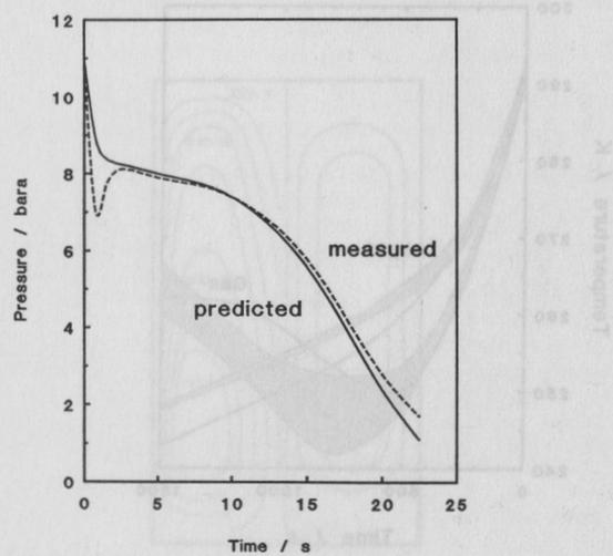
Figure 8 Pressure at intact end of LPG line
