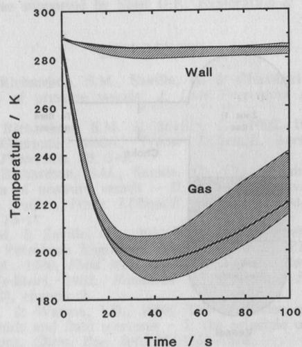
Figure 3 Bulk gas and inside wall temperatures in vessel A: hatched regions span experimental measurements, solid lines are predictions
