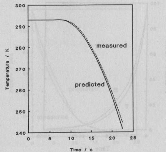
Figure 9 Temperature at intact end of LPG line
