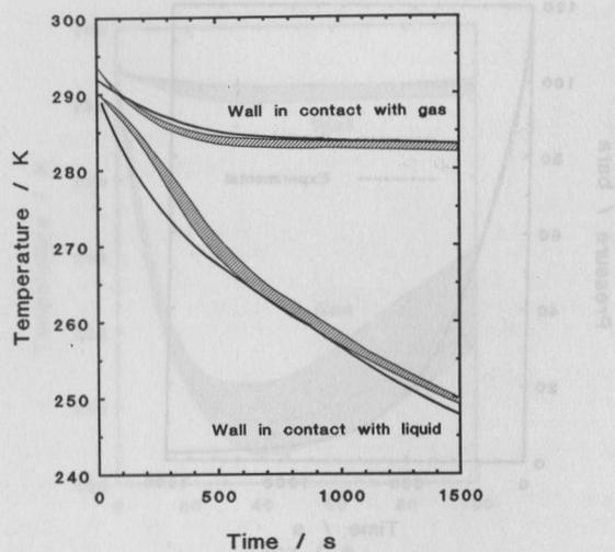
Figure 7 Inside wall temperatures in vessel B: hatched regions span experimental measurements, solid lines are predictions
