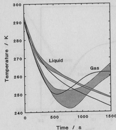
Figure 6 Bulk gas and bulk liquid temperatures in vessel B: hatched regions span experimental measurements, solid lines are predictions
