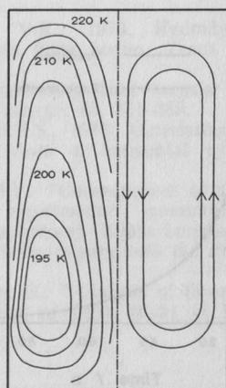
Figure 4 Isotherms (left-hand side) and schematic streamlines (right-hand side) in vessel A: horizontal scale is exaggerated for clarity
