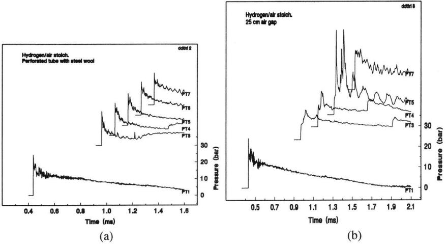
Figure 11. Pressure histories for a hydrogen-air detonation showing (a) transmission and (b) transition to detonation when the perforated mesh is replaced by a 25 cm long air gap.
