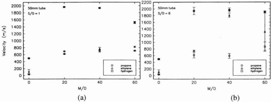
Figure 7. Measured shock-flame front velocity just prior to the arrester as a function of accelerating section length ( $M/D$ ) for two obstacle spacings; Disks spaced (a) one diameter and (b) six diameters apart.
