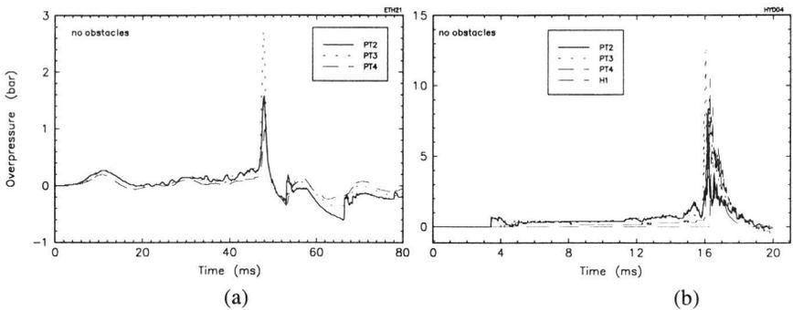
Figure 4. Pressure time histories at various gauge locations showing the pressure evolution in a 50 mm tube without an accelerating section, (a) ethylene- and b) hydrogen-air.
