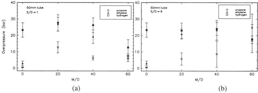
Figure 8. Measured peak overpressure just prior to the arrester as a function of accelerating section length ( $M/D$ ) for two obstacle spacings, (a) one and (b) six diameters apart.
