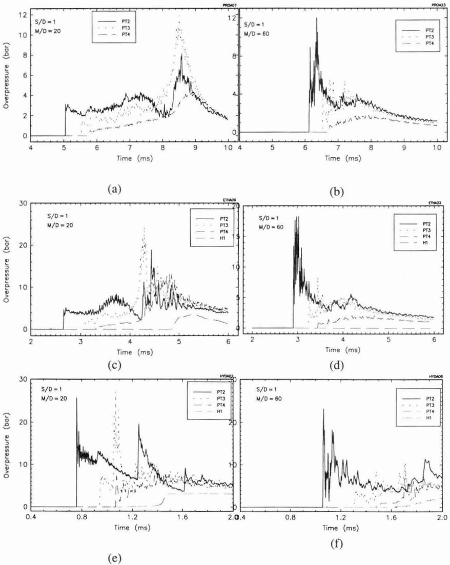
Figure 5. Pressure evolution and light emission downstream of the arrester (H1) for an obstacle spacing of 1 pipe diameter ( $S/D$ ) and two lengths of accelerating section ( $M/D$ ) for propane (a and b), ethylene (c and d) and hydrogen (e and f).
