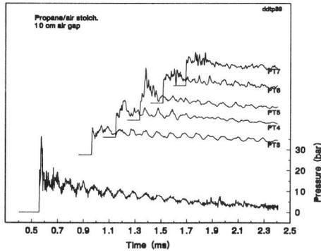
Figure 9. Pressure histories obtained for a propane-air detonation incident on a 10 cm air gap, showing the failure to re-initiate.
