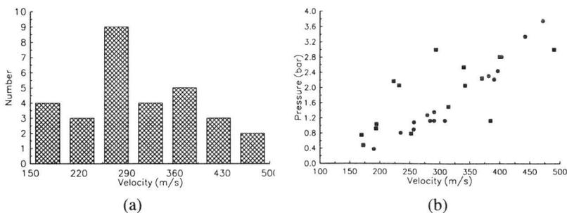
Figure 1. Graphs showing variations in (a) measured velocities and (b) correlation between pressure and velocity, both obtained for essentially constant initial conditions.
