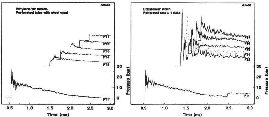
Figure 10. Pressure histories for an ethylene-air detonation showing failure (left) and transition to detonation (right) when a series of disks are introduced downstream of the attenuator.
