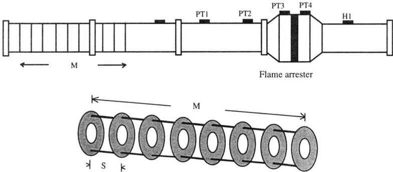
Figure 2. Schematic of basic flame acceleration test configuration
