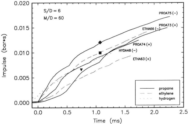
Figure 12. Plot showing impulse time histories for different mixtures for an accelerator section with an obstacle spacing  $S/D = 6$  and overall length  $M/D = 60$ . Solid symbols indicate the time at which arrester failure is first observed.
