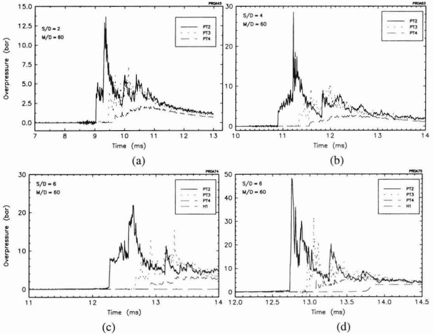
Figure 6. Pressure histories obtained with the maximum length of accelerating section ( $M/D=60$ ) for a range of obstacle separations ( $S/D$ ). The mixture is propane-air. (c) and (d) are repeat test showing incipient DDT and an actual transition to detonation.
