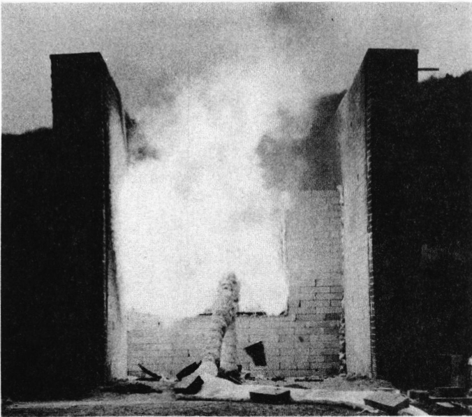
Figure 3 (b). Propane vapour jet fire engulfment
