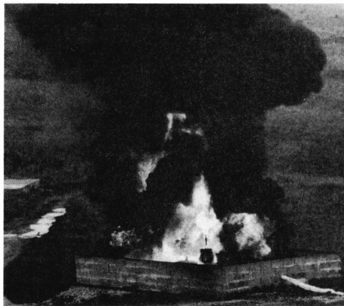
Figure 1(b). Pool fire engulfment
