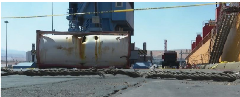
Figure 5 – Puncture holes in ISO container
