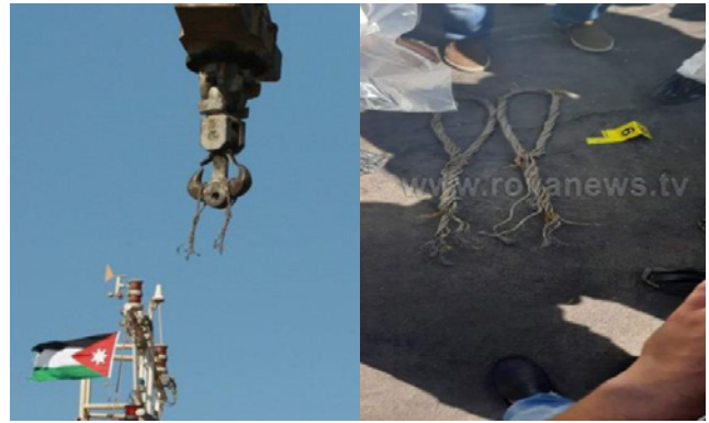
Figure 6 – Lifting wire failure
