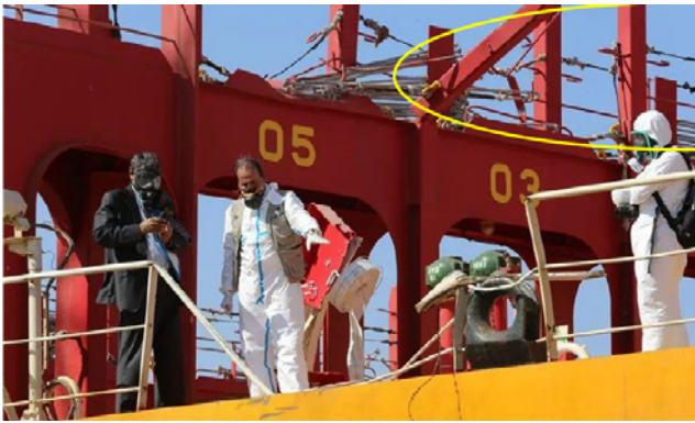
Figure 4 – Damage to cell guides (circled) and railing
