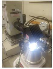
for controlled light exposure during reactions. It is rated for operation up to 8 bar and 200 °C, making it suitable for investigating low-pressure hydrogenation and dehydrogenation processes. Illumination is provided by a xenon (Xe) arc lamp, with filters applied to remove ultraviolet (UV, <420 nm) and infrared (IR) wavelengths. This ensures that only visible light contributes to the reaction, enabling precise evaluation of lightdriven catalytic effects.
