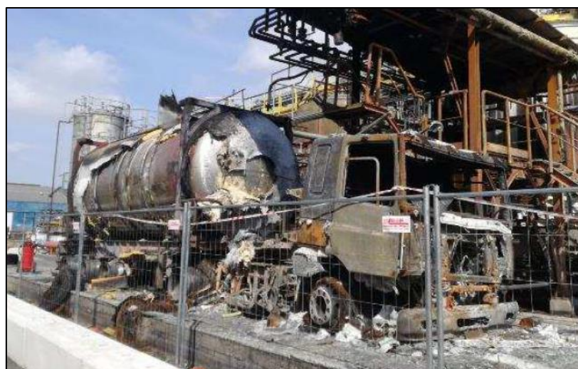
Fig. 6. Consequences on equipment and structures: Tanker Truck
