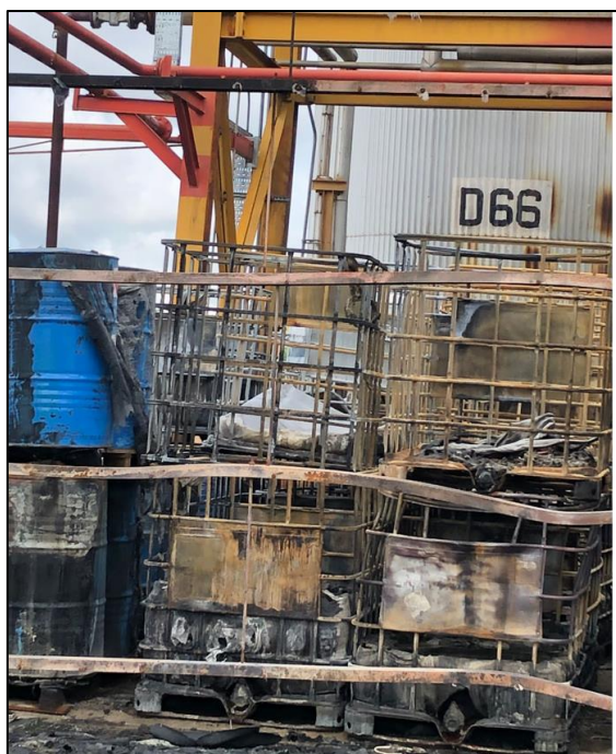
Fig. 6. Consequences on equipment and structures: IBC and DRUMS
