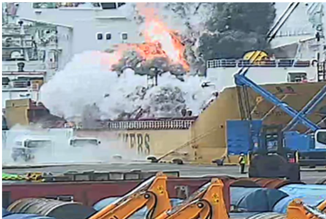
Figure 2: Ignition of styrene vapour after thermal runaway caused overpressurisation of the cargo tank
