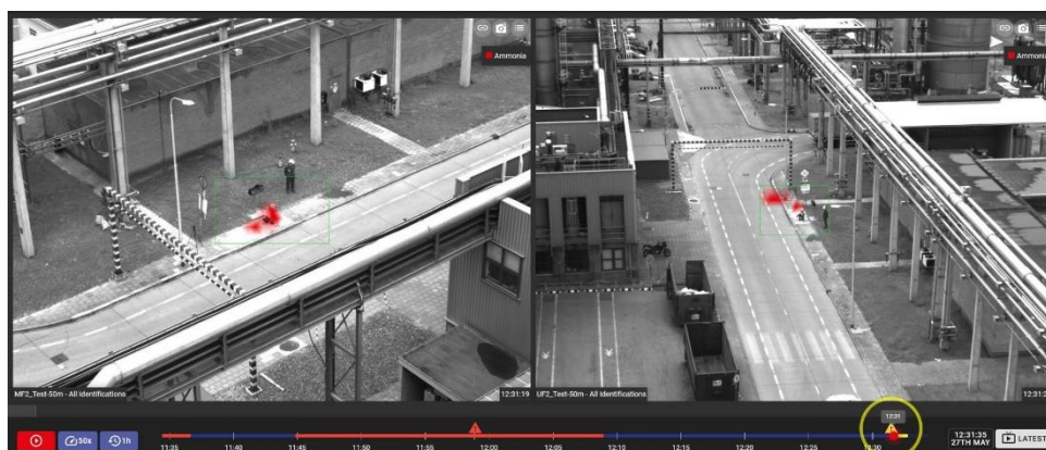
Figure 8 Small scale release experiment with ~100 ml of 25% ammonia water in an open container. To sensor units capture the area and the Profiler identifies a „Low Alert“ (yellow triangle in the timeline).
