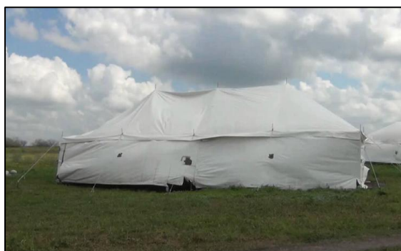
Figure 9: Experimental Tent Response to a Given Load
