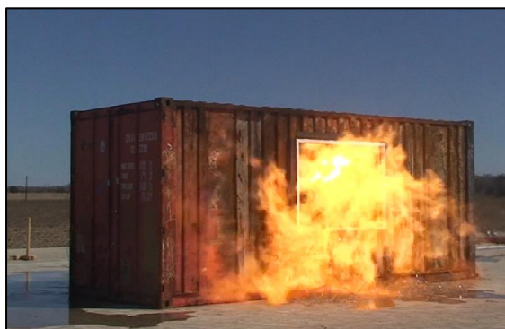
Figure 13: External View of Jet Fire Impingement on BRM with Window
