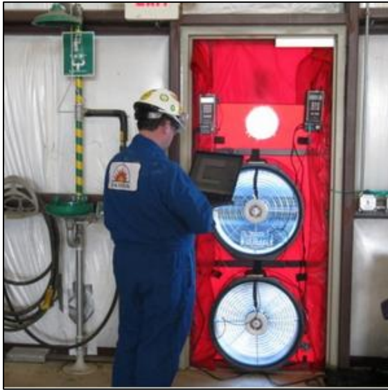
Figure 15: A Blower Door Test for Gas Ingression
