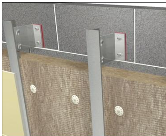
Figure 21: Rockwall Thermal Barrier on Wall Inside
