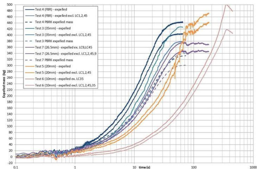
**Figure 8. Expelled mass – effect of hole diameter (with insulation; tests 4,3,7,5,6)**
