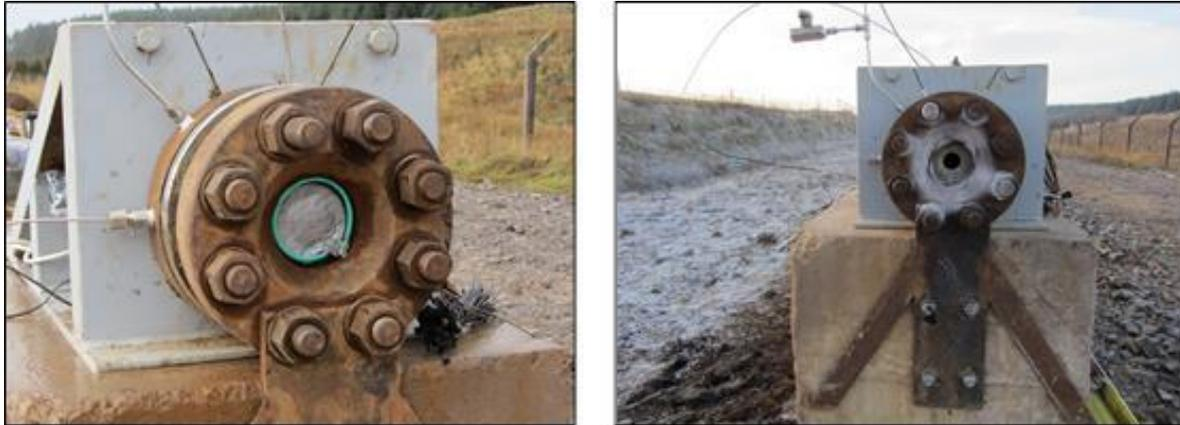
**Figure 3. Bursting Disc Before and After a Test**
