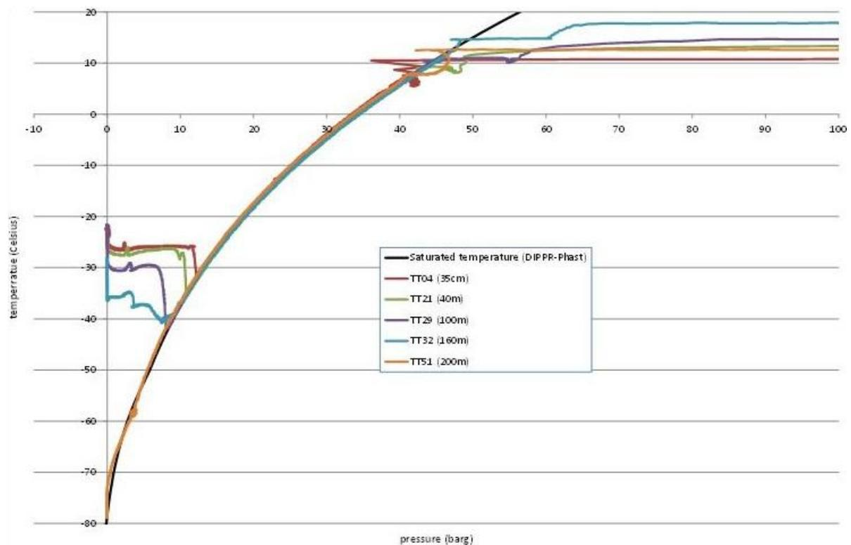
(b) measured temperature versus pressure
