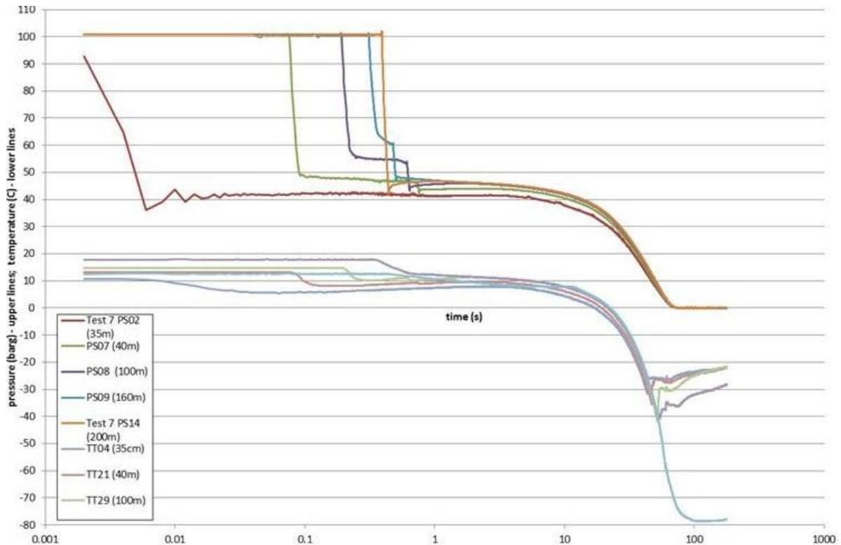
(a) measured pressure and temperature versus time
