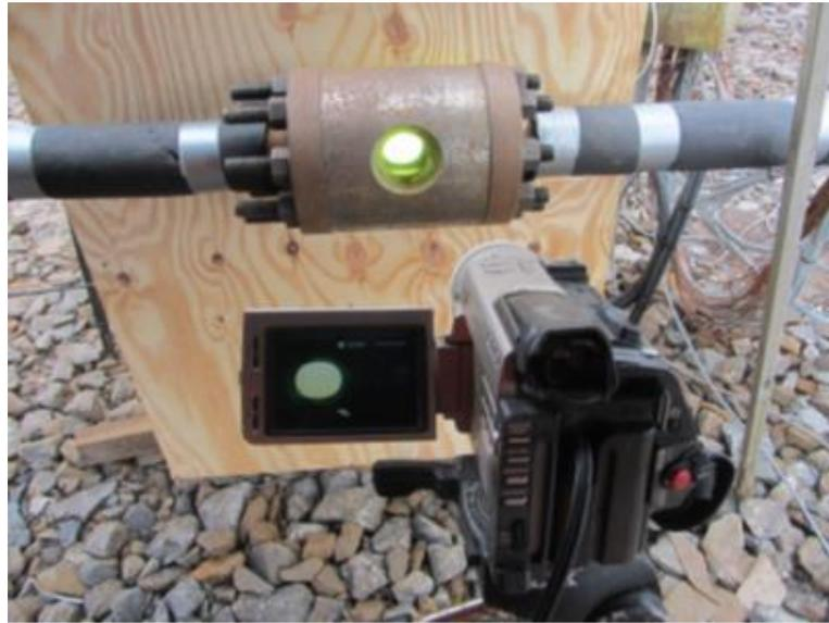
**Figure 4. Viewing Window Mid-Length Along Pipe**
