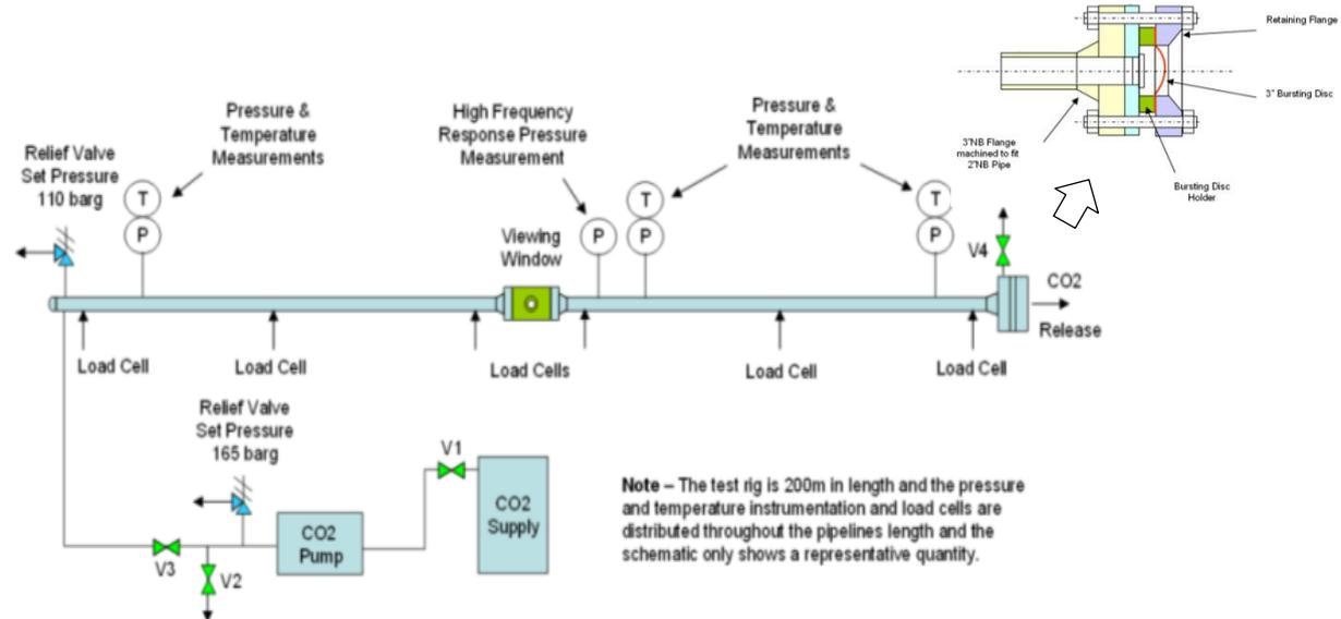
**Figure 1. Schematic Layout of Test Facility**
