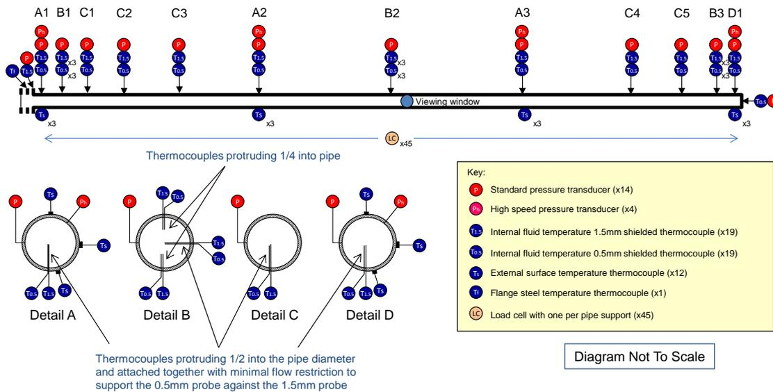
**Figure 5. Shock Tube Instrumentation Schematic**
