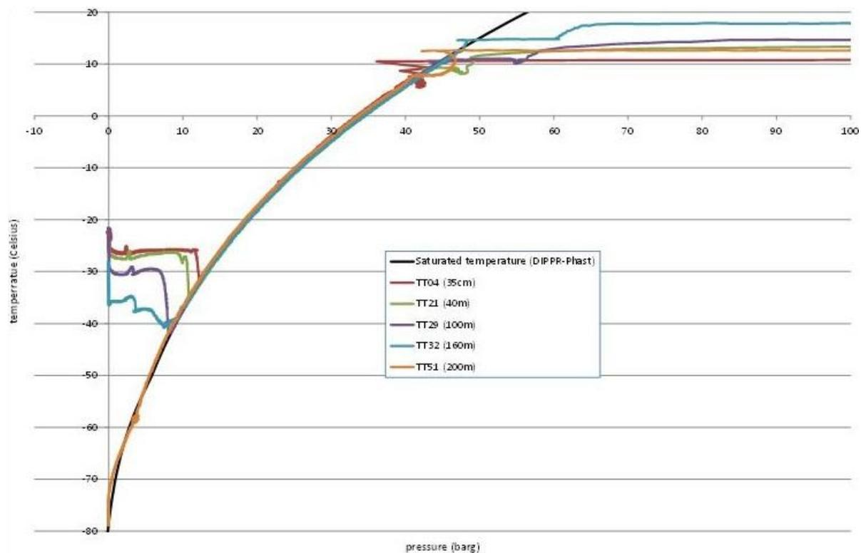
(b) measured temperature versus pressure
