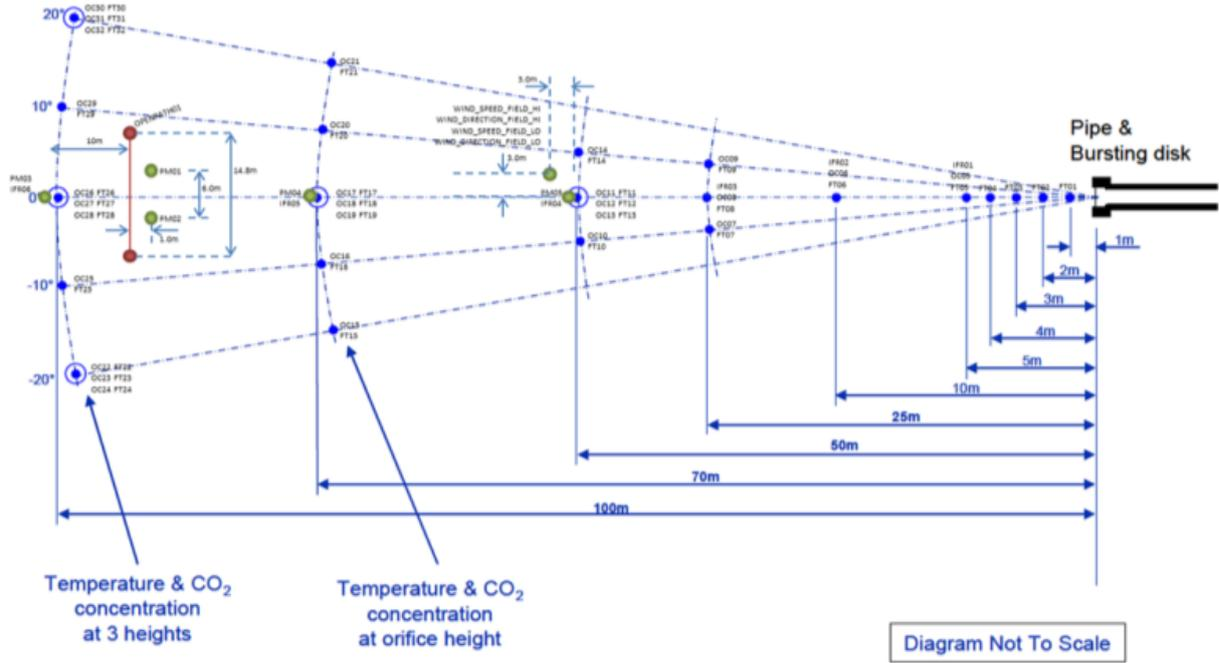
Figure 7. Indicative Field Instrument Array
