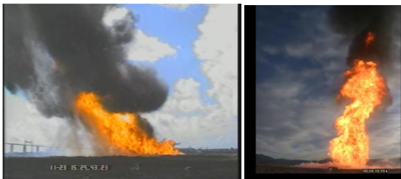
Figure 6 : The Montoir LNG pool fire tests (left) show a greater production of smoke than the SNL experiment (right).
