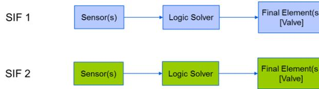
In Figure 14, separate logic solvers are shown for the two functions. However, if the two functions (SIF1 and SIF2) are intended to provide an overall level of risk reduction of, say 200, then this would be equivalent to a single function with a performance<sup>13</sup> in the range for Safety Integrity Level (SIL) 2. Therefore, the two functions could utilise the same logic solver provided it has been designed as suitable for SIL 2 operation.
