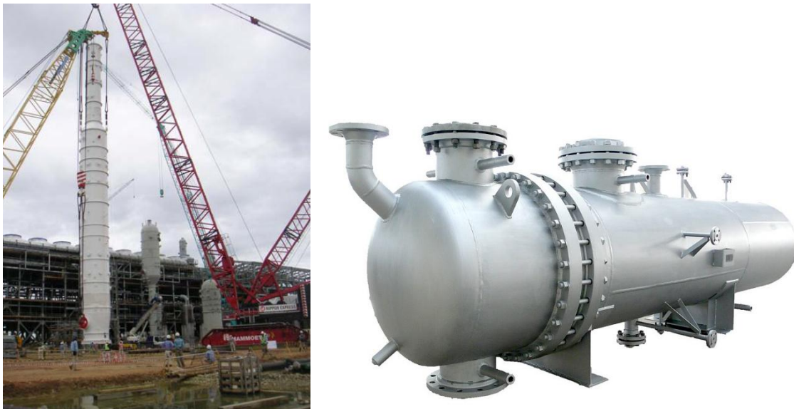
Figure 1 – Comparison in size and fittings of a MCHE (left) and S&T HE (right)
