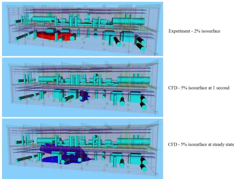
Figure 9. A31 – Experimental Results in Red and CFD in Blue
