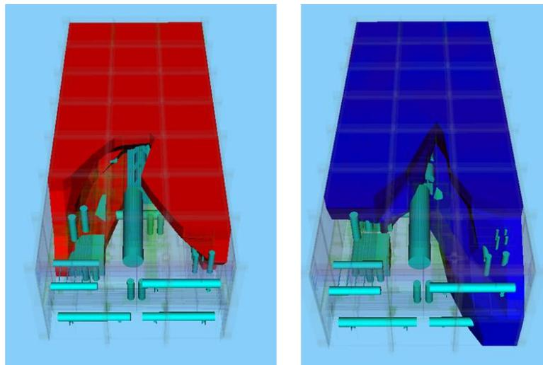
Figure 8. A12– Experiment on the Left (Red), CFD on the Right (Blue)
