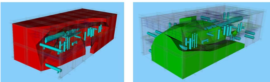
Figure 14. C17 – Experimental Results in Red and CFD in Green using 10.5m/s Wind and Refined Grid in Wake of the Module (ALFL)
