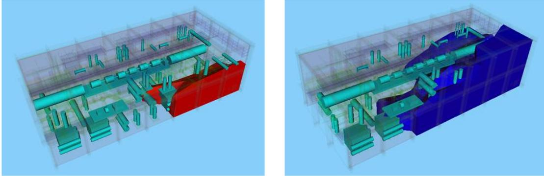
Figure 6. A30 – Experiment on the Left (Red), CFD on the Right (Blue)
