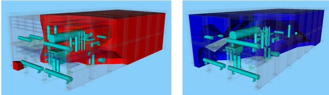
Figure 11. C12 – Experimental Results in Red and CFD in Blue (ALFL)
