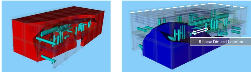
Figure 12. C17 – Experimental Results in Red and CFD in Blue (ALFL)
