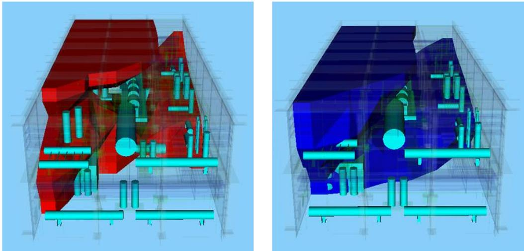
Figure 7. A15– Experiment on the Left (Red), CFD on the Right (Blue)
