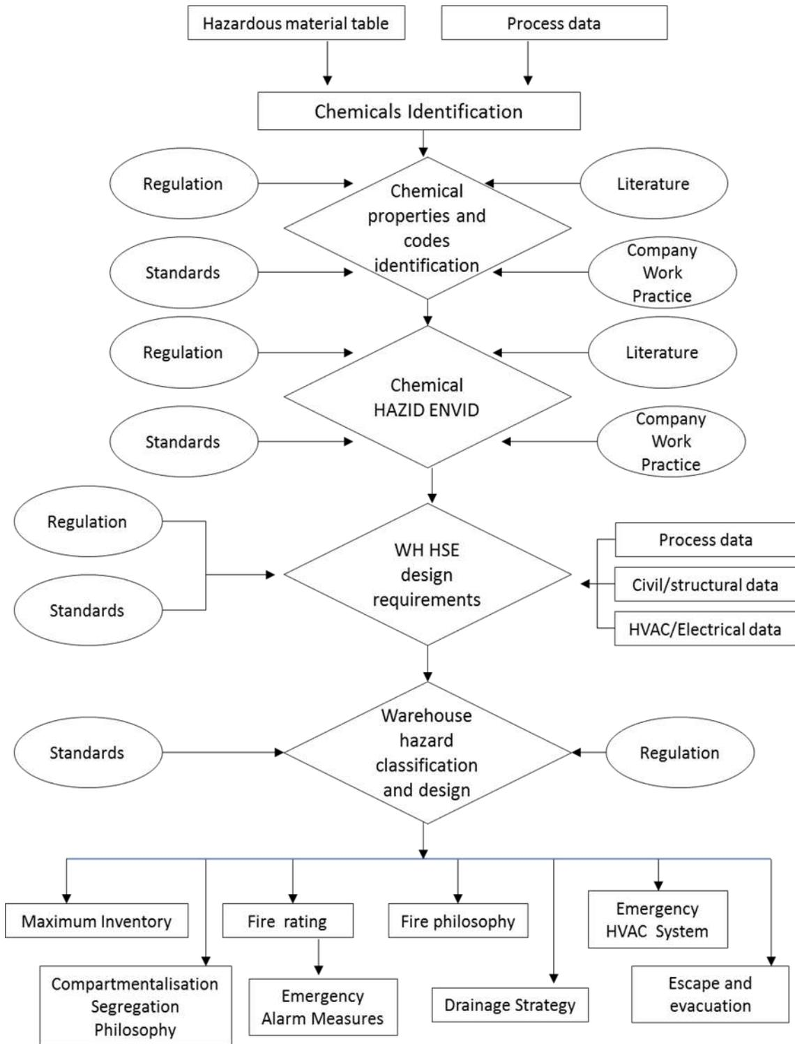
Figure 1: Warehouse safe design flow-chart
