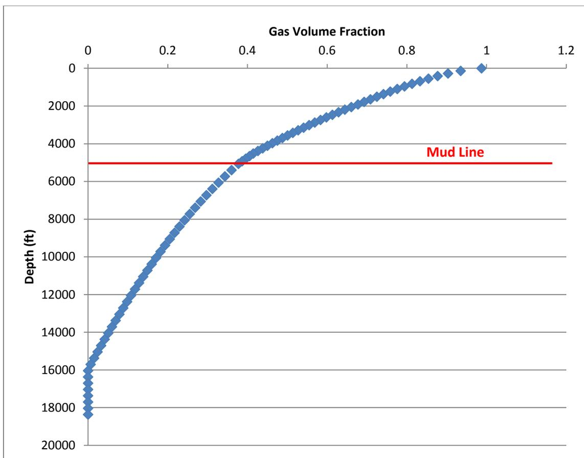
Figure 4. Gas volume fraction along the wellbore
