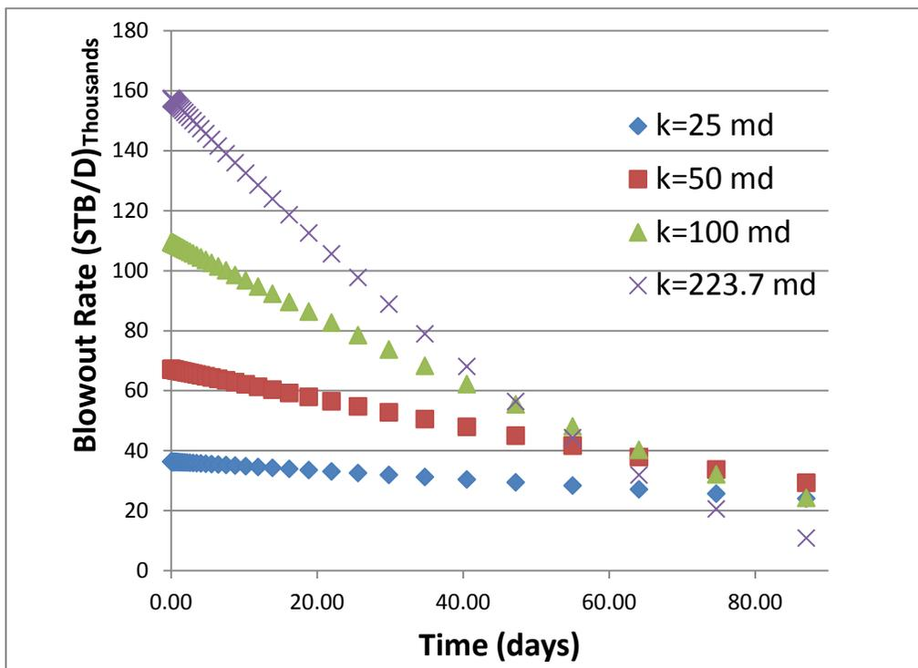
Figure 2. Blowout rate evolution with different permeability
