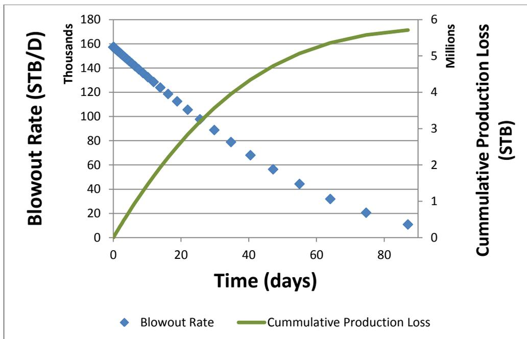
Figure 1. Simulated blowout rate and cumulative production loss during Macondo incident
