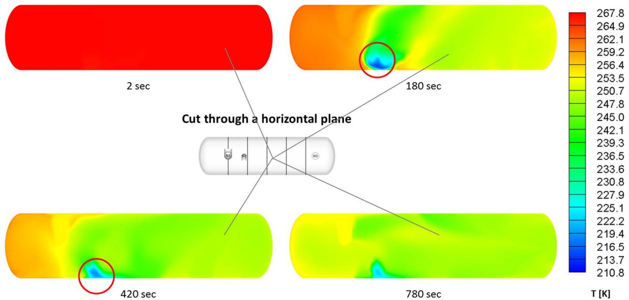
**Figure 8.** Temperatures of fluid from CFD analysis
