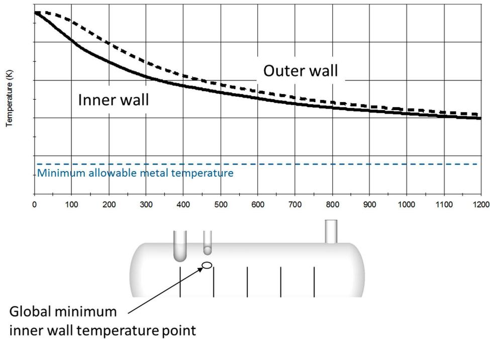
Figure 10. Wall temperatures from hybrid analysis
