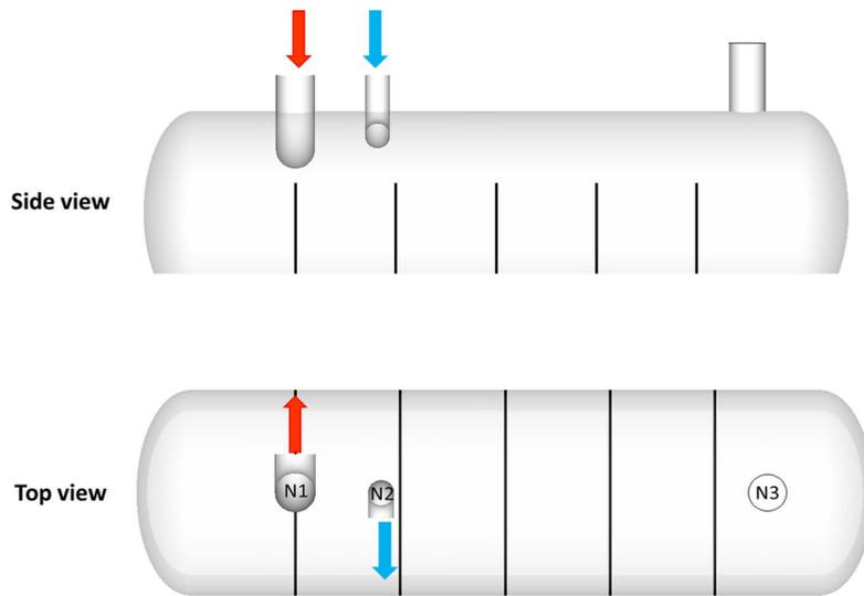
Figure 6. Oil-gas separator inlet flows through nozzles: side and top views
