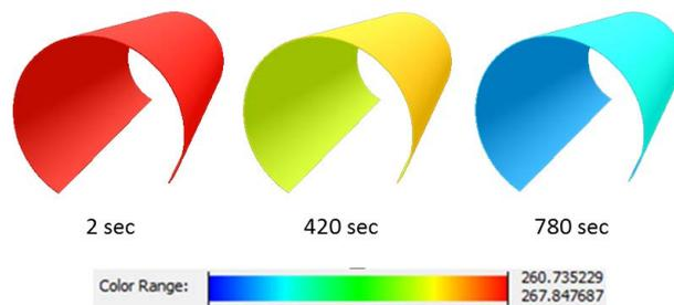
**Figure 5.** ‘Lumped’ approach results, showing uniform temperatures throughout the separator walls
