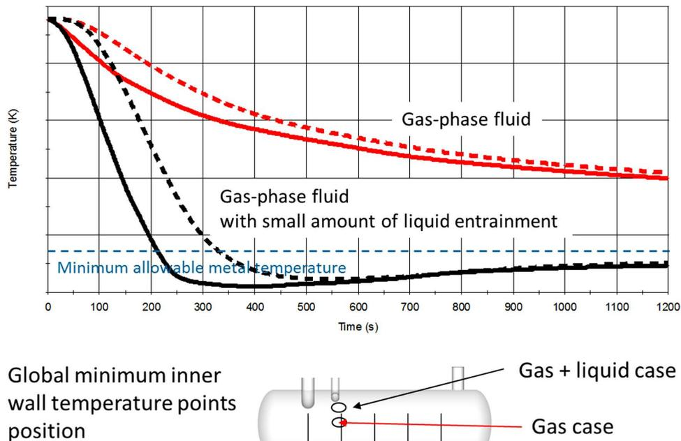
Figure 11. Hybrid model separator global minimum wall temperatures over time for gas-only (red) and entrained liquid (black) cases. Dotted and solid lines represent outer and inner wall temperatures respectively
