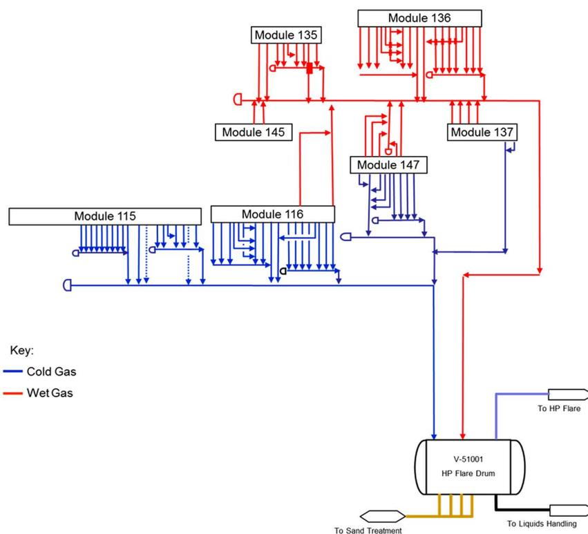
Figure 1. Example configuration: HP Flare system KO drum
