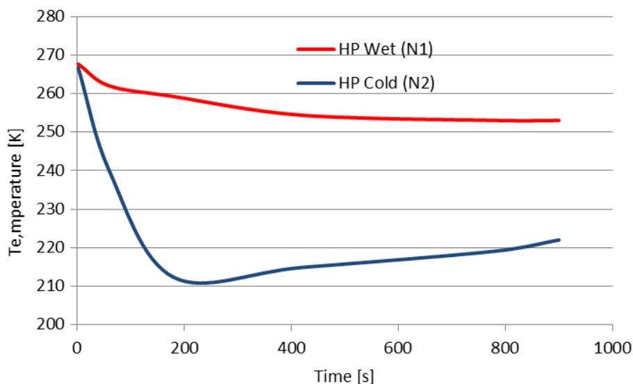
**Figure 3.** Temperatures of entering flows
