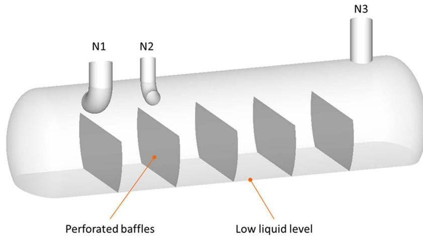
**Figure 2.** Typical HP Flare system KO drum configuration
