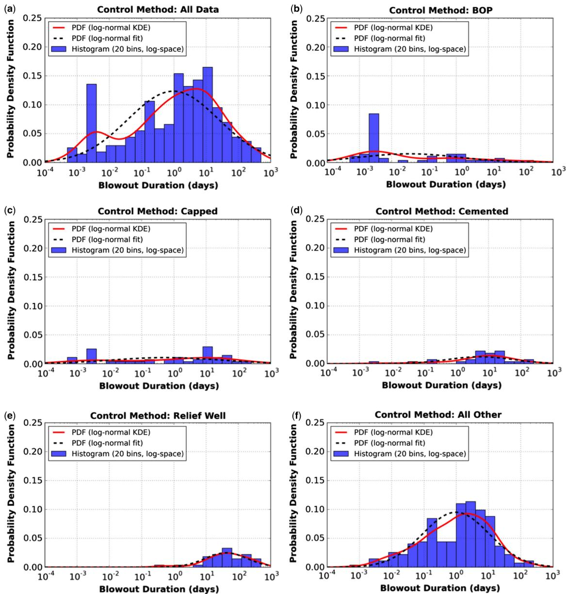
**Figure 1.** Probability density functions for historical blowout durations, split by control method. All curves/histograms have been weighted by the total number of points for all control methods
