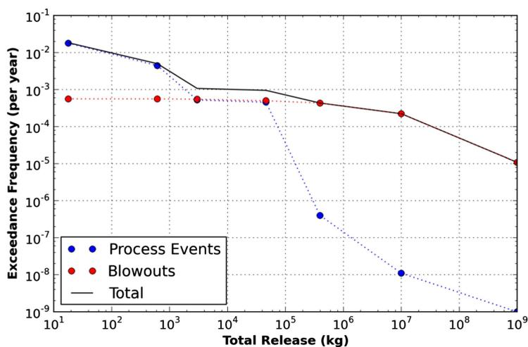
**Figure 5.** Example combined mass released exceedance curve for process and blowout events.
