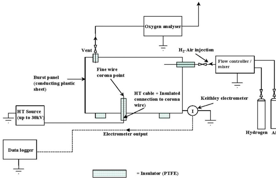
**Figure 4.** Schematic of the experimental arrangement used for ignition of H<sub>2</sub>-Air mixtures from generated corona discharges
