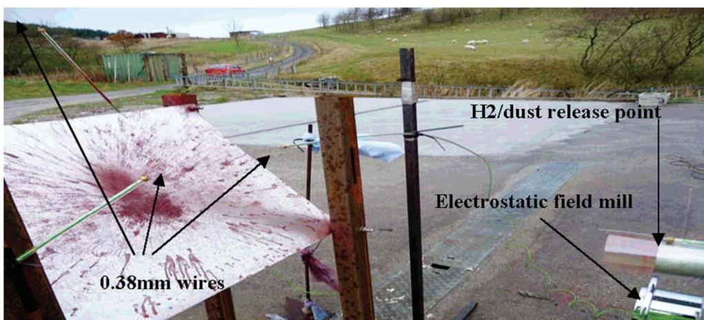
**Figure 8.** Arrangement to investigate electrostatic field/discharges during hydrogen release and dust dispersion
