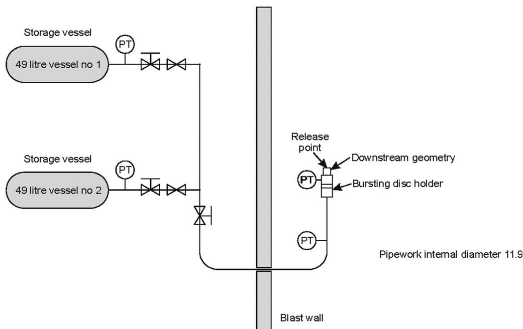
**Figure 2.** Simplified schematic of the spontaneous ignition high-pressure H<sub>2</sub> test facility
