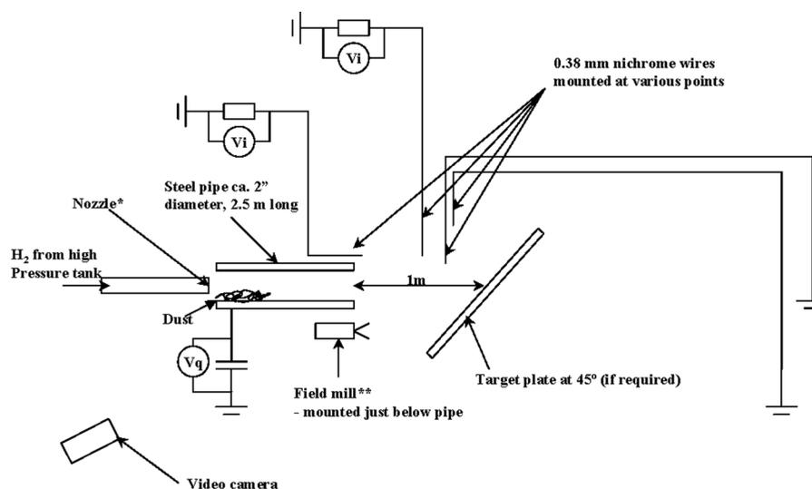
\* Internal orifice plates can be fitted to change the hydrogen flow rate
