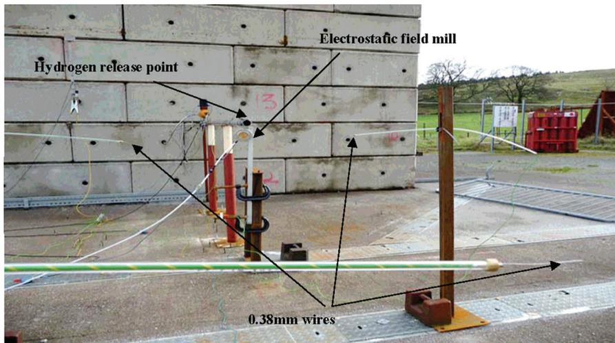
**Figure 7.** Arrangement to investigate electrostatic field/discharges during hydrogen release
