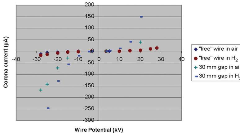
**Figure 5.** Corona current versus potential applied to the wire electrode
