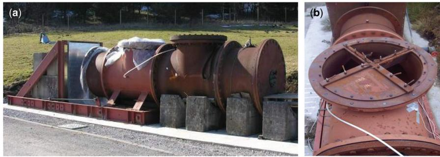
**Figure 2.** Photograph of (a) the 1.04 m diameter explosion vessel and (b) the  $\frac{3}{4}$  open relief vent
