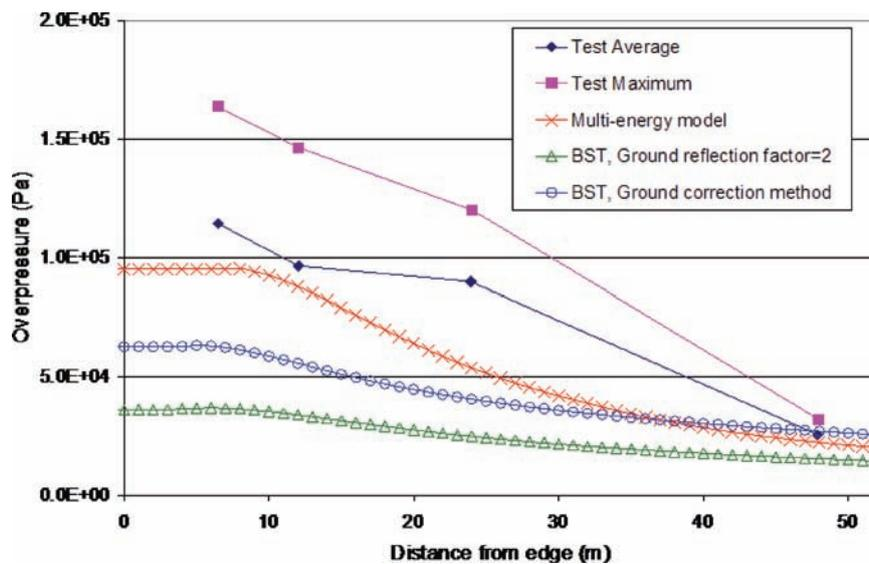
Figure 5. Comparing the overpressures along a transect crossing the explosion source (BFETS3a\_B)
