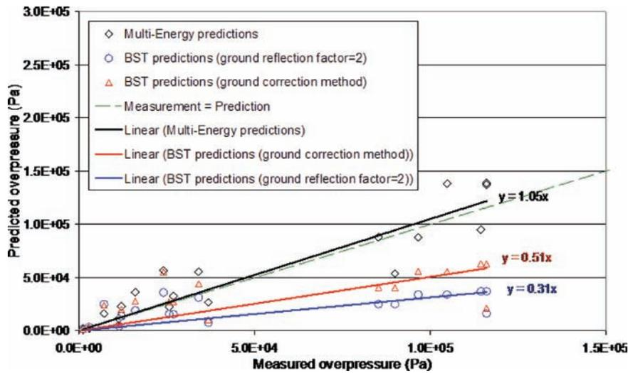
Figure 4. Comparing the overpressure predictions of BST and multi-energy models against measurements (selected cases)
