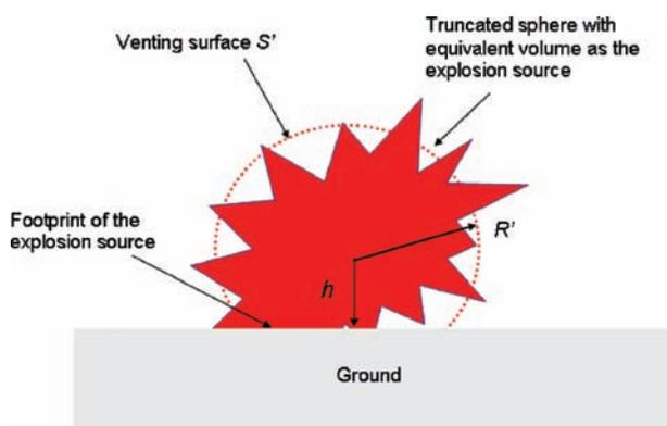
**Figure 2.** An elevated vapour cloud explosion and the representation by a truncated sphere
