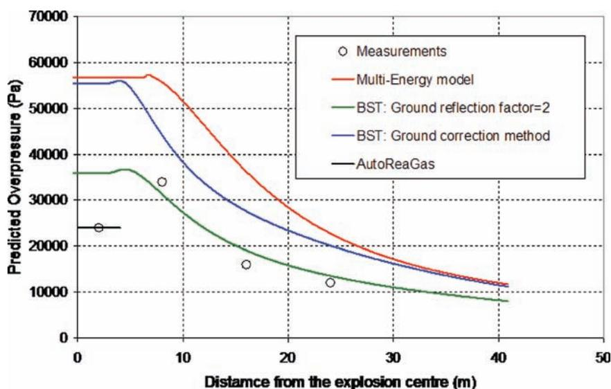
**Figure 6.** Comparing the overpressures along a transect crossing the explosion source (The gas processing case of the GAMES study)
