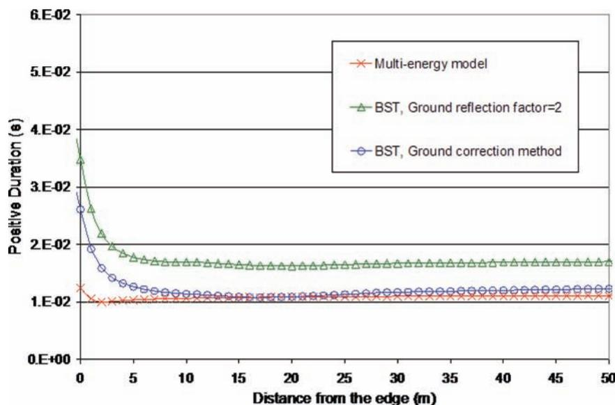
**Figure 7.** Comparing the predicted positive duration along a transect crossing the explosion source (EMERGE6)
