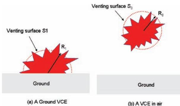
Figure 1. Ground and air vapour cloud explosions (VCEs)
