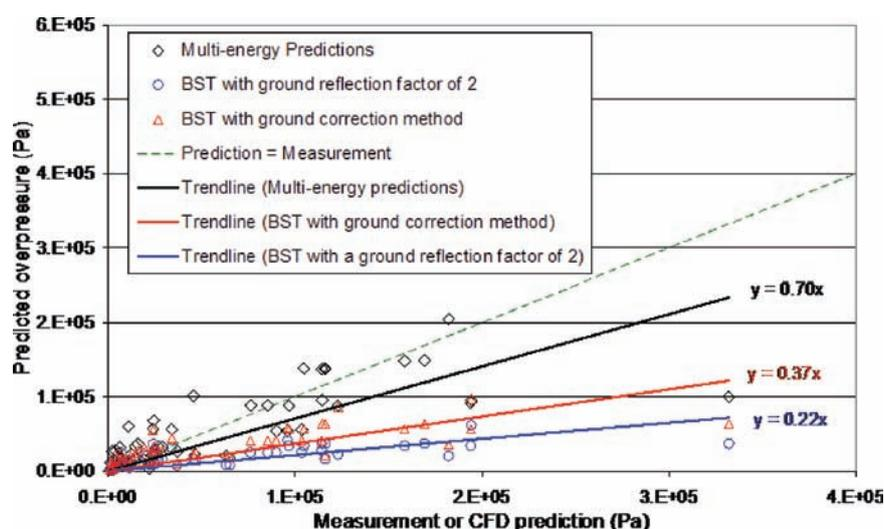
**Figure 3.** Comparing the overpressure predictions of BST and multi-energy models against measurements and CFD predictions (all cases)
