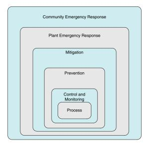
Prevention – process alarms with mandatory operator corrective actions, safety instrumented control systems and safety instrumented protective systems. These devices are designed to return the process to a safe state if it moves outside the normal operating limits.
