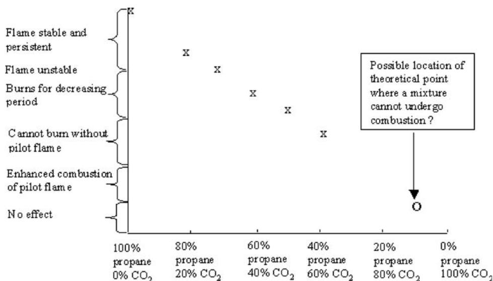
**Figure 4.** Illustrative graph showing changes in combustion stability as a function of propane/CO<sub>2</sub> concentrations
