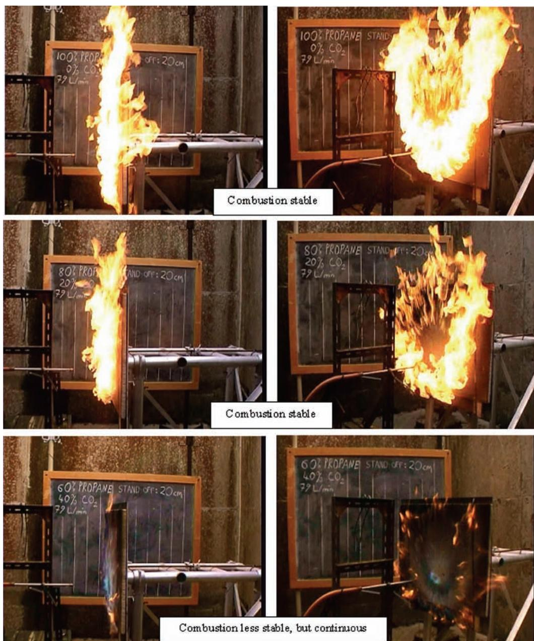
**Figure 3.** Effects of flame impingement on combustion in ignited propane/CO<sub>2</sub> mixtures of differing ratios. Nozzle – plate separation 20 cm, flow rate 79 l.s<sup>-1</sup>
