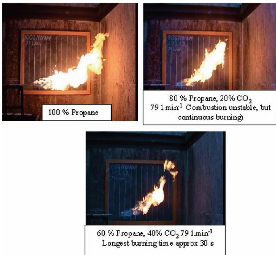
**Figure 2.** General appearance of flames from ignited propane/CO<sub>2</sub> mixtures of differing ratios. Flow rate 79 l.s<sup>-1</sup>
