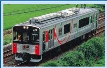
2006, Japan World's first Hydrogen train 2 x 95 kW fuel cells
