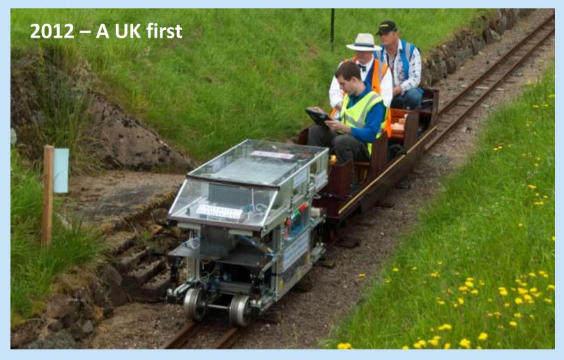
University of Birmingham's Hydrogen locomotive powered by a 1kW fuel cell at the IMechE's Railway Challenge on the Stapleford 10 ¼ inch miniature railway 1<sup>st</sup> July 2012
