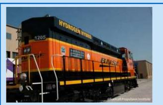
2010, Los Angeles, USA 130-ton diesel shunter 240 kW fuel cell
