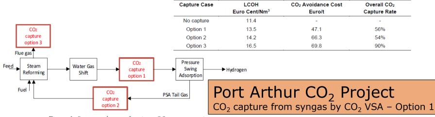
Figure 1: Steam methane reforming - CO<sub>2</sub> capture options
