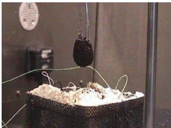
**Figure 7.** Sub critical behaviour depicted by a localised charring around the hotspot
