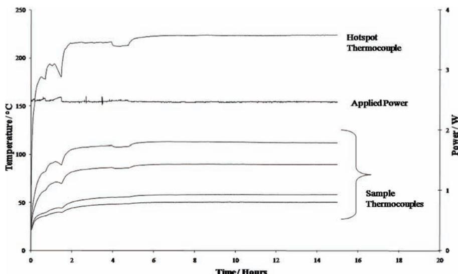
Figure 4. Typical experimental trace for a no ignition test in carbon
