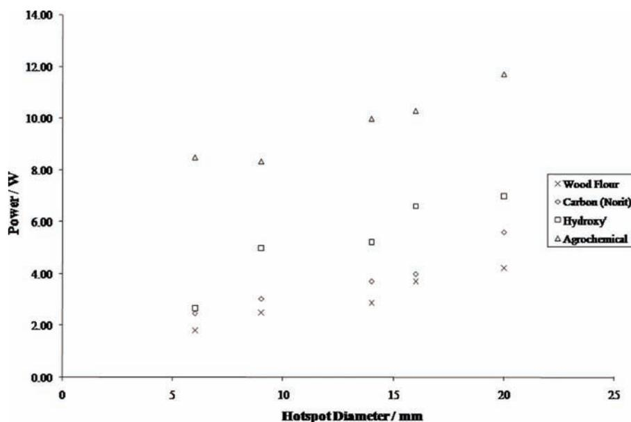
Figure 9. Relationship between the lowest measured critical power and hotspot size for each material studied
