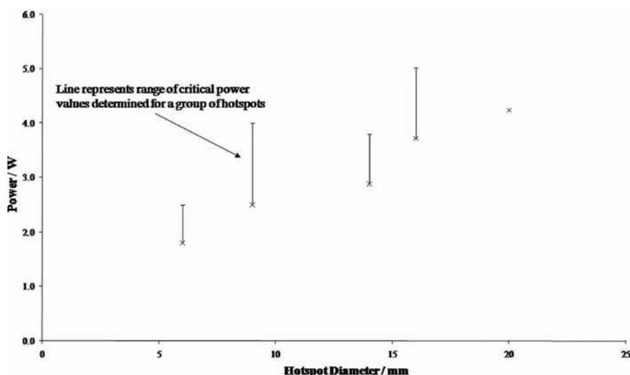
Figure 3. Critical power determined in wood flour
