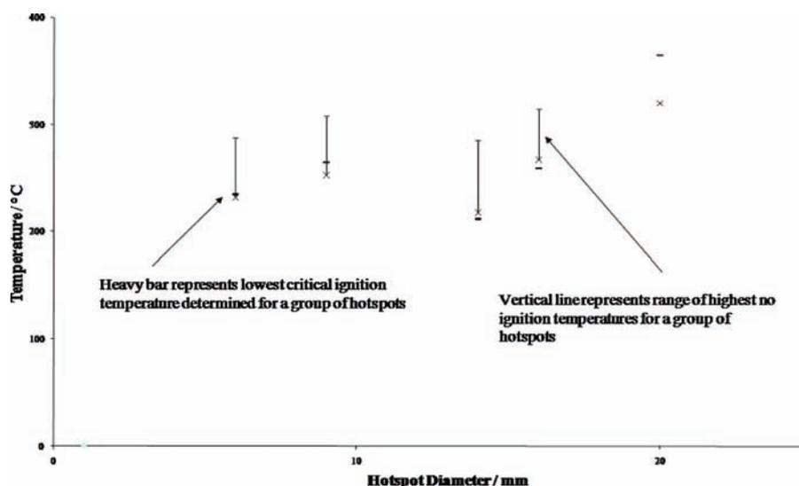
Figure 6. Range of no ignition temperature and lowest critical ignition temperature determined in wood flour
