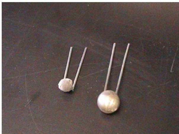
Figure 2. Hotspot design – moulded ceramic sphere on the left, brass sphere on the right
