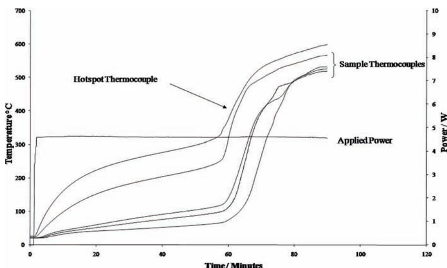
Figure 5. Typical experimental trace for an ignition test in wood flour
