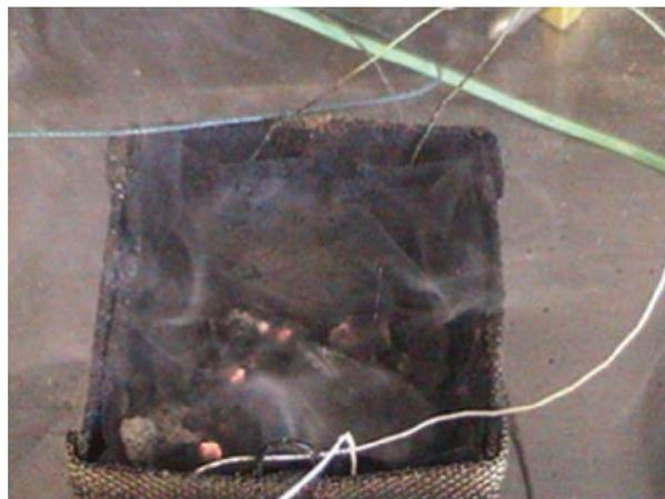
**Figure 8.** Critical behaviour depicted by ignition and smouldering combustion/decomposition of the test material
