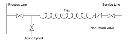
The best place for the blow-off point is at the process end as then it can be used to prove that the hose is clear, by opening the service and blow-off valves before the process vale is opened.
