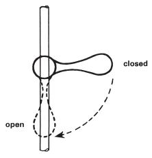
To prevent this happening the valves should be installed so that when they are open the valve handle points upwards.
