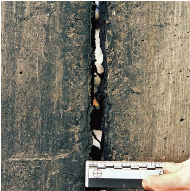
**Figure 5.** Buncefield. Loss of integrity at a bund expansion joint
