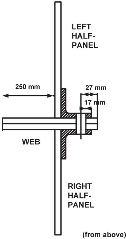
Figure 2. Half-Panel and Web Assembly
