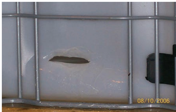
Figure 3. IBC pierced by fork lift truck
