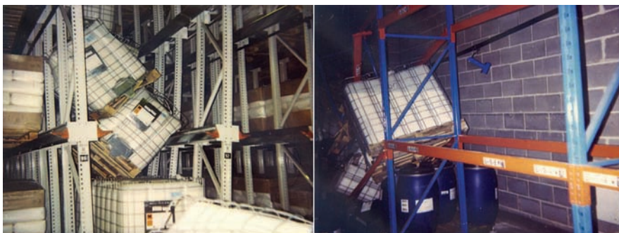
Figure 2. Racking collapse incident
